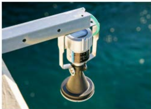
Figure 23. The Hydra-Pulse 235 radar water level sensor.
