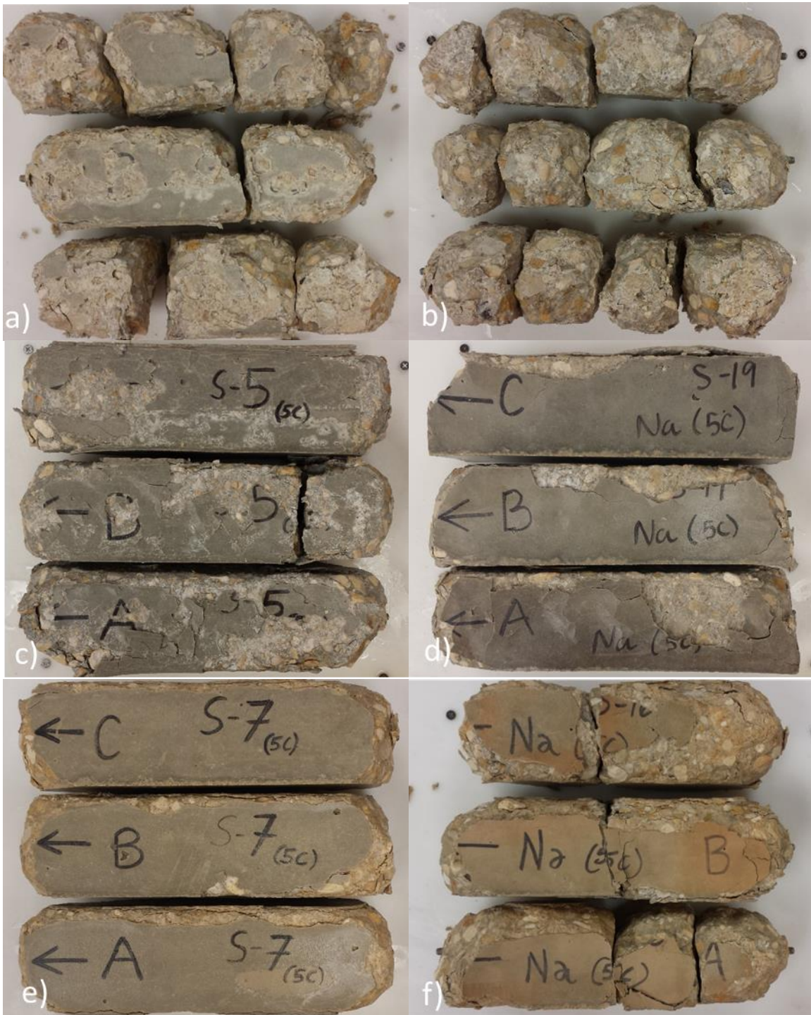
a) PLC3+20%C1 after 15 months, b) PLC3+20%C2 after 18 months, c) PLC3+20%C1+5%SF after 18 months, d) PLC3+20%C2+5%SF after 18 months, e) PLC3+40%C1 after 18 months f) PLC3+40%C2 after 18 months.
