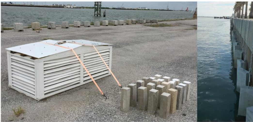
Figure 7.2: Carbonation and ASR Exposure Sites (left) and Corrosion Specimens Hanging from Seawall (right)
