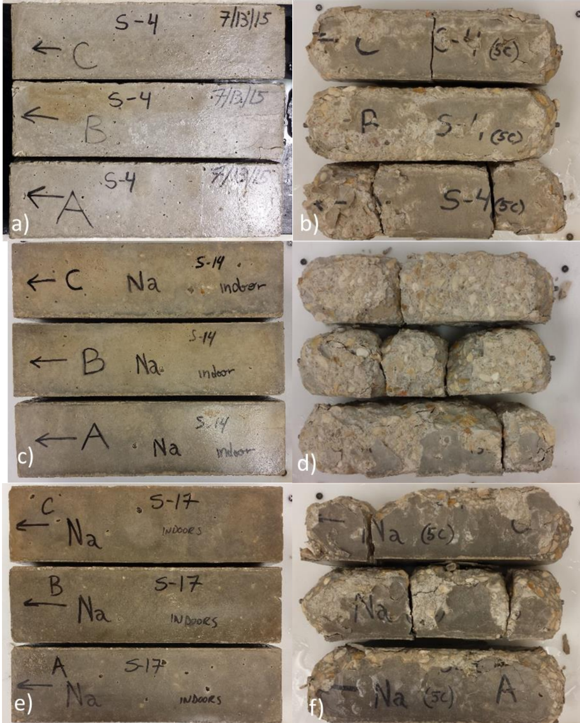
a) PLC3 at 23°C, b) PLC3 at 5°C, c) PLC4 at 23°C, d) PLC4 at 5°C, e) PLC7 at 23°C, f) PLC7 at 5°C. Figure 10.14: Concrete Specimens with 20% Class F Fly Ash Stored in Laboratory Conditions after 18 Months of Exposure
