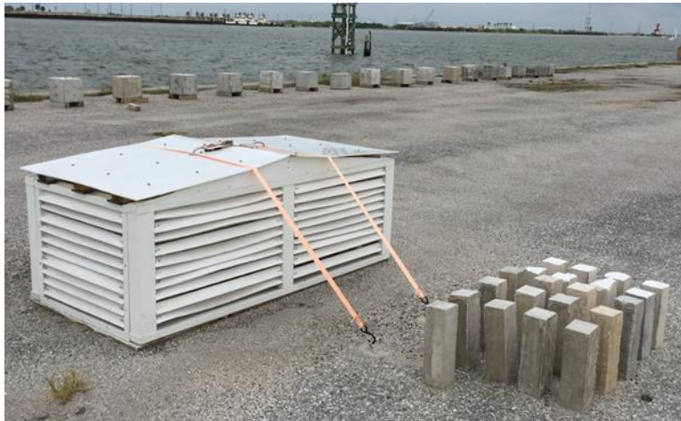
Figure 8.5: Carbonation Exposure Site on the Gulf Coast
