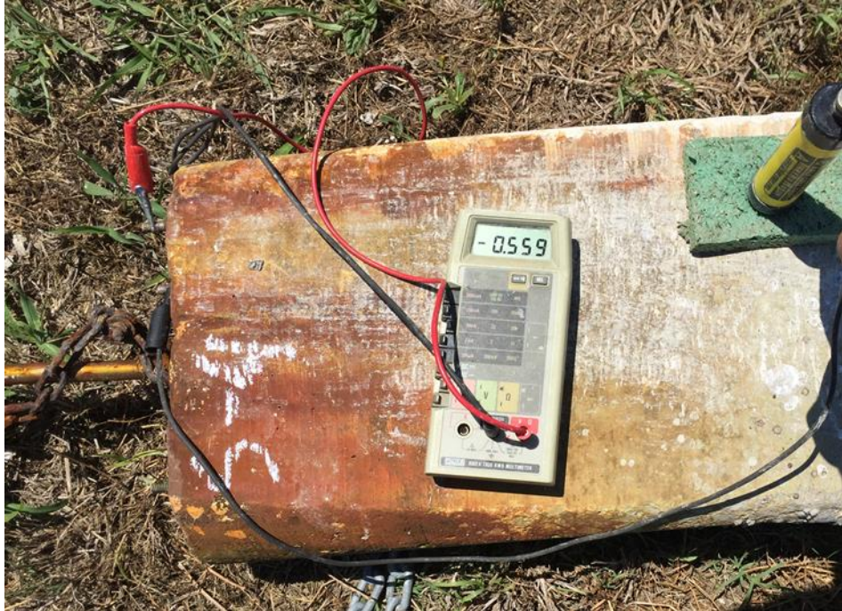
Figure 7.5: Half-Cell Potential Measurement Procedure
