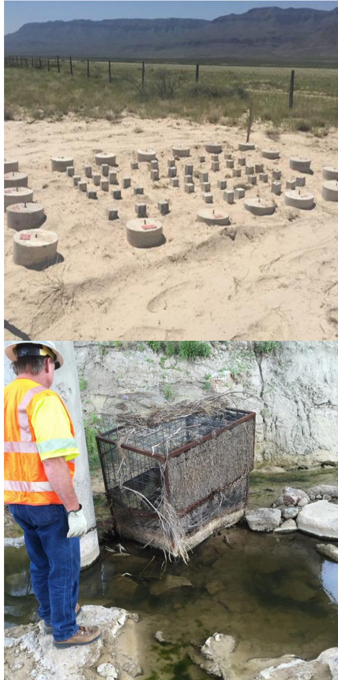
Figure 10.3: Exposure Sites near Van Horn, TX in Areas of Calcium Sulfate Soil
