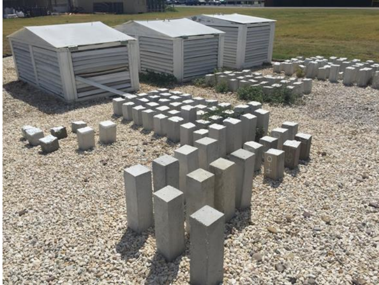
Figure 8.4: Carbonation Exposure Site in Austin, TX
