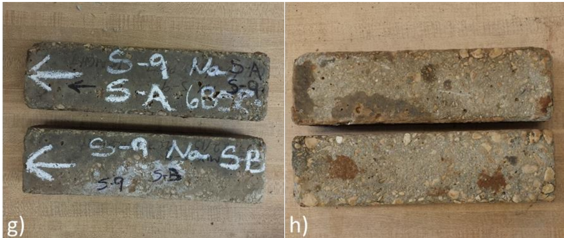
a) PLC1 after 15 months, b) PLC2 after 16 months, c) PLC3 after 24 months, d) PLC4 after 24 months, e) PLC5 after 24 months, f) PLC6 after 24 months, g) PLC7 after 24 months, h) Type V after 24 months.
