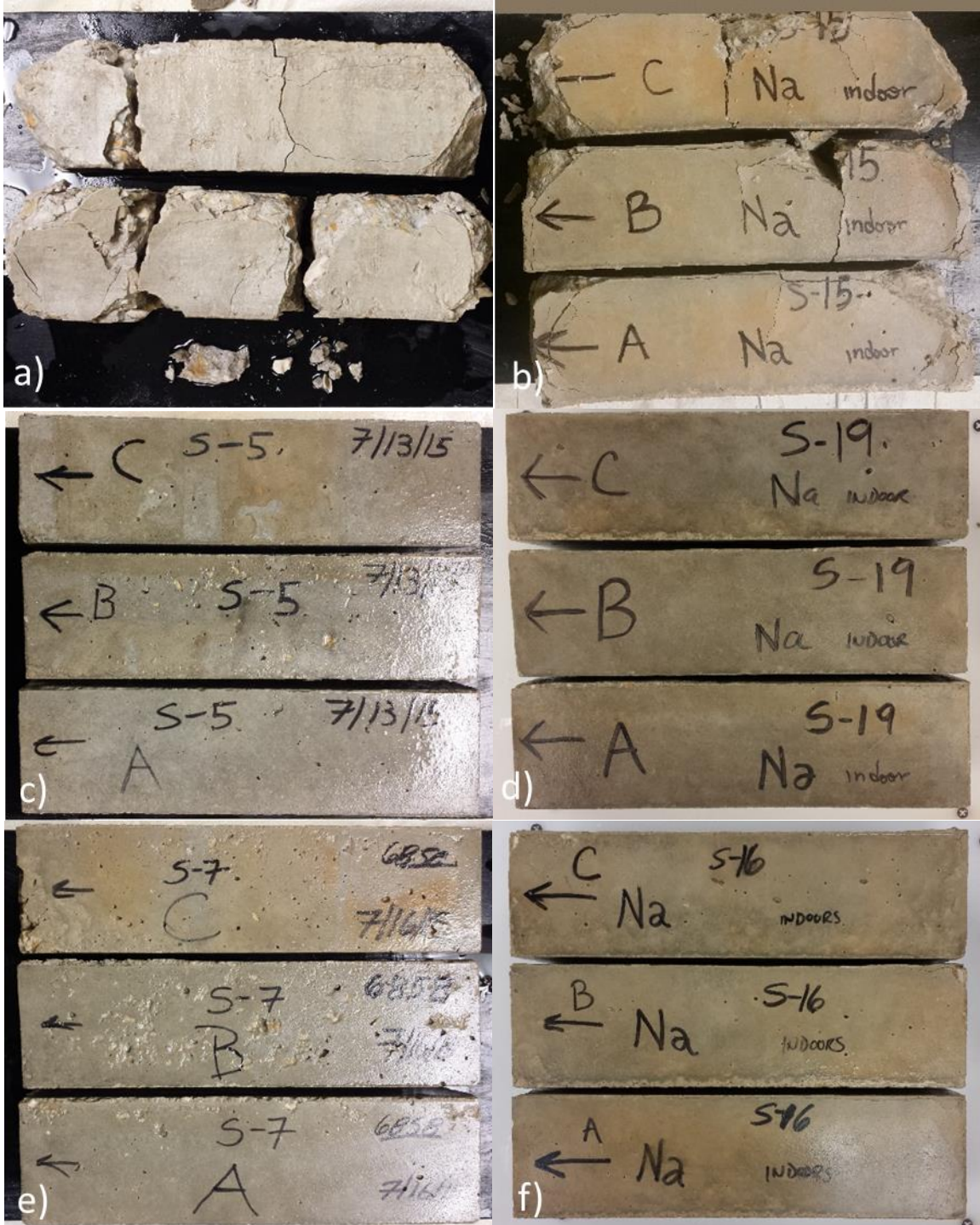
a) PLC3+20%C1 after 24 months, b) PLC3+20%C2 after 15 months, c) PLC3+20%C1+5%SF after 24 months, d) PLC3+20%C2+5%SF after 24 months, e) PLC3+40%C1 after 24 months, f) PLC3+40%C2 after 24 months.
