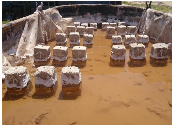
Figure 10.2: Partially Submerged Concrete Prisms in \text{Na}_2\text{SO}_4 Outdoor Exposure Site
