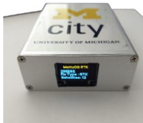
Figure 33: Mcity's RTK unit for pedestrians and cyclists.
