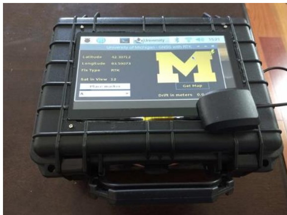
Figure 32: Mcity's RTK unit for vehicles.
