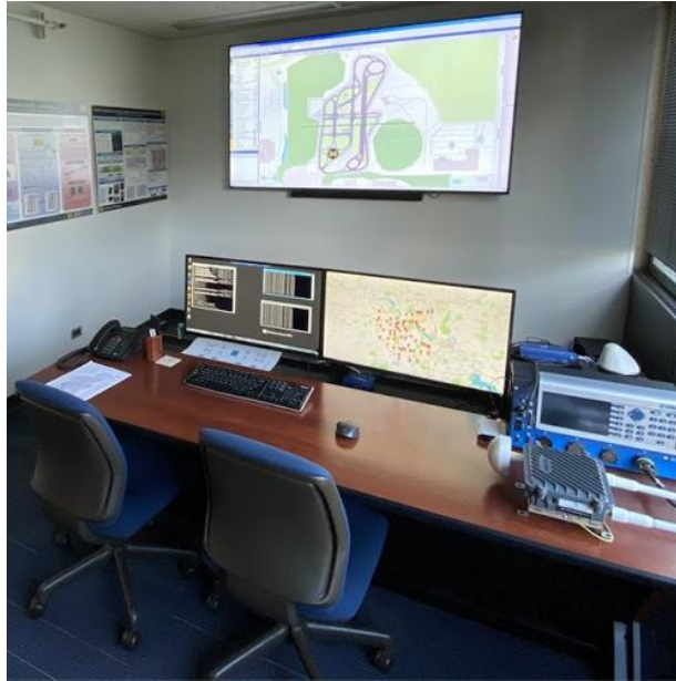
Figure 5: Mcity Traffic Management Center, which is also linked to the City of Ann Arbor traffic control network at 70+ signalized intersections and specialized roadside installations – overlaid on the lower right-hand display.
