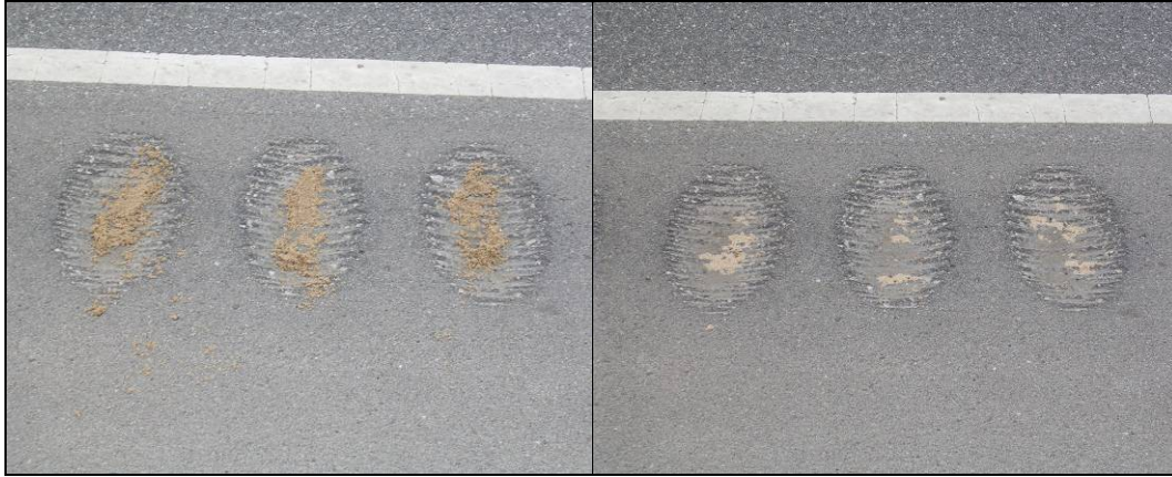
Figure 4.4: Football Rumble Strips, Debris Test Trial 2 at time = 0 hr. (left) and at time = 18 hrs. (right).
