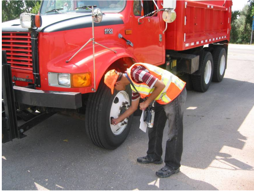
Figure 4.19: Measuring the air pressure on the 1996 International 4900 DT 466 Dump Truck
