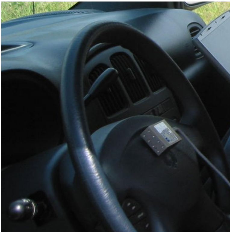
Figure A13: Summit Instruments accelerometer attached to steering wheel, vibration test setup
