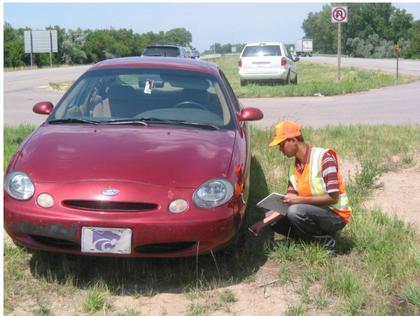
Figure 4.20: Measuring the air pressure on the 1996 Ford Taurus LX
