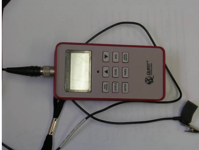
Figure 4.11: Quest Technologies Q-300 Noise Dosimeter with an external microphone
