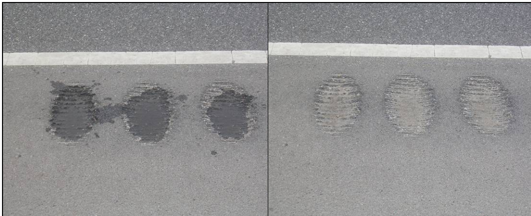
Figure 4.8: Football Rumble Strips, Water Test Trial 2 at time = 0 hr. (left) and at time = 18 hrs. (right).
