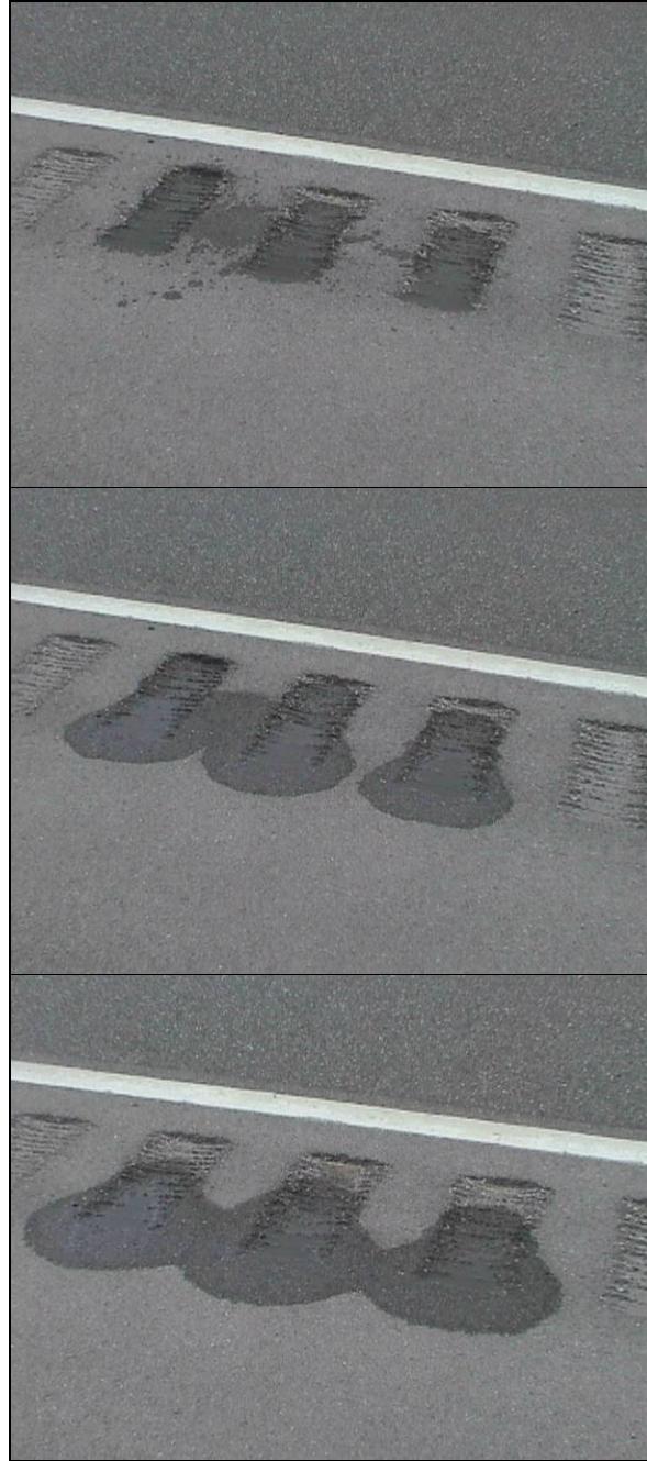
Figure 4.9: Rectangular Rumble Strips, Water Test Trial 3 at time = 0 min. (top), at time = 45 min. (middle), and at time = 90 min. (bottom).
