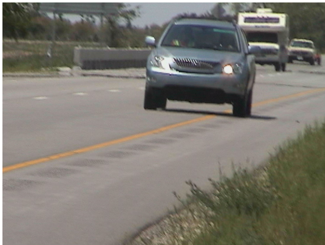
Figure 4.14: 2005 Lexus RX300 Sport Utility Vehicle crossing football shaped rumble strips
