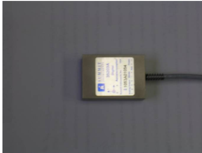
Figure 4.15: Summit Instruments 35203A Digital Accelerometer
