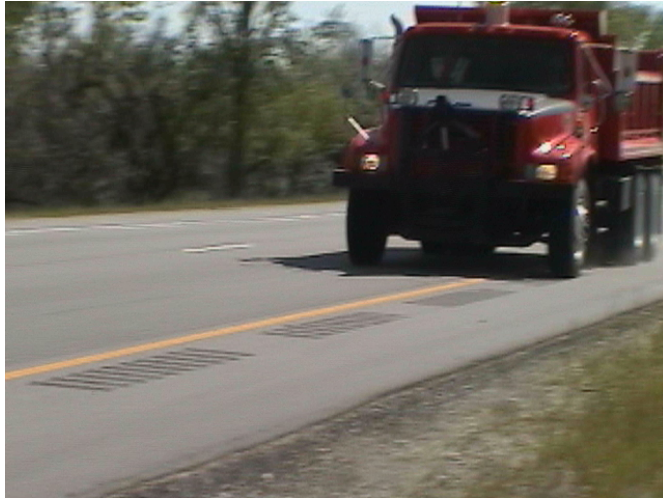
Figure 4.12: 1996 International 4900 DT466 Dump Truck crossing rectangular rumble strips
