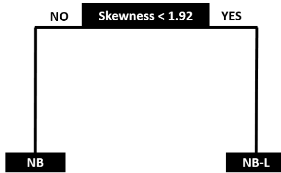
Fig. 4: Heuristic for Model Selection between the NB and NB-L Distributions. (Note: tree can be used for data with 0.1 < \text{mean} < 20 and 1 < \text{VMR} < 100 )
