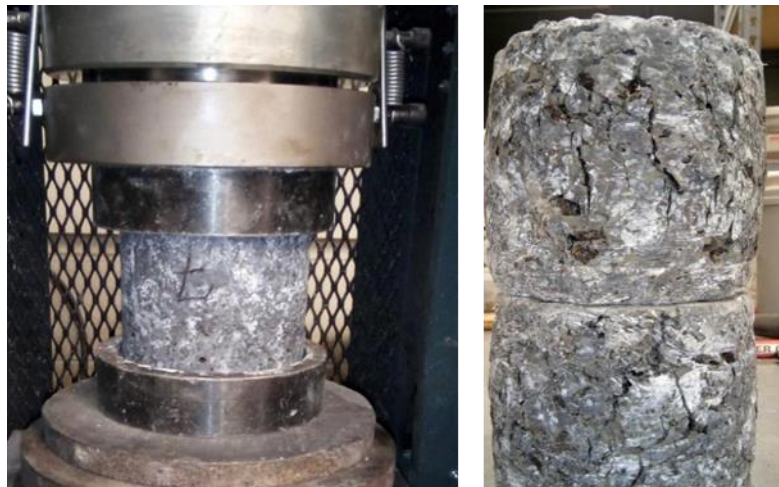
Figure 4.2. Compressive strength test and failed samples
