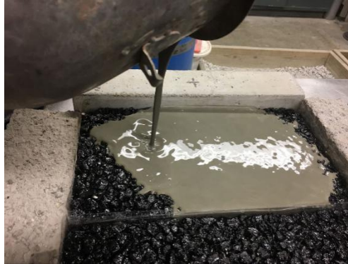
(b) Pouring grouting materials
