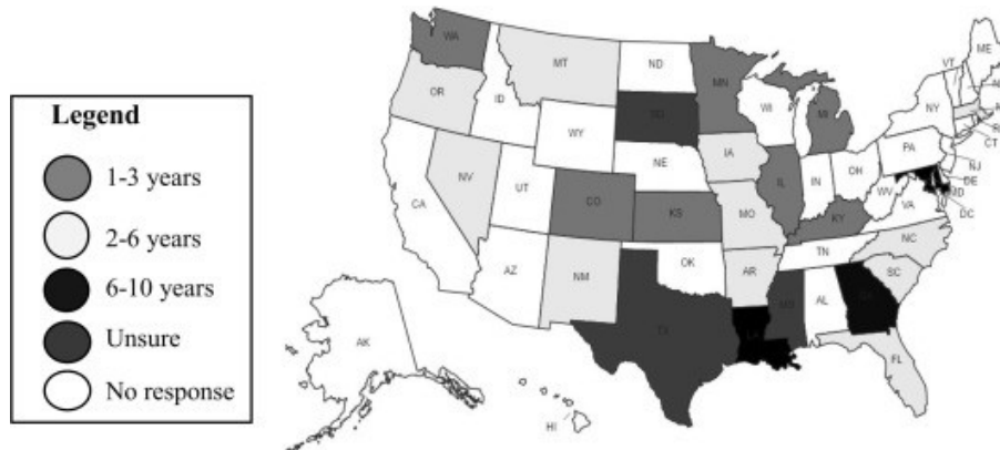
Figure 3. The average service life of an HMA overlay against reflection cracking (1).
