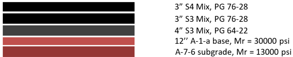
Fig. 4.10 Case Study Flexible Pavement Structure
