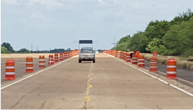
Figure 1. Overview of the experimental environment. Each roadside had 44 barrels spaced about 20 m (or 60 feet) apart.
