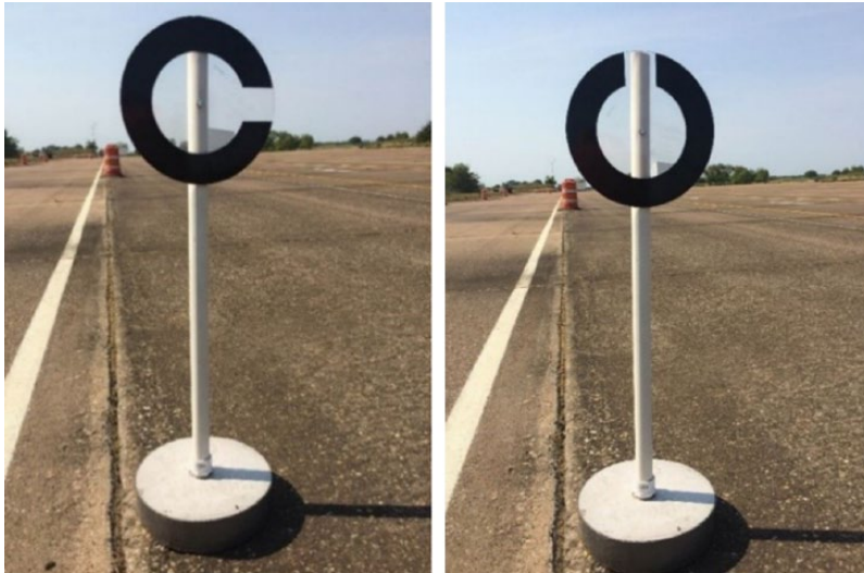
Figure 5. Experimental signage (Left: “C” orientation, Right: “U” orientation). The “C” orientation signified a need to C hange lanes following a verbal response, whereas the “U” orientation required a verbal response only (“lane should be U nchanged”). The post heights were adjusted to be as tall as the TDBs so the post and the affixed sign can be obscured in distance. The signage was made in two sizes: 10-in. and 6-in. diameter. Eight signs on each roadside included four pairs of 10-in. and 6-in. signs, alternating the large and small sizes.
