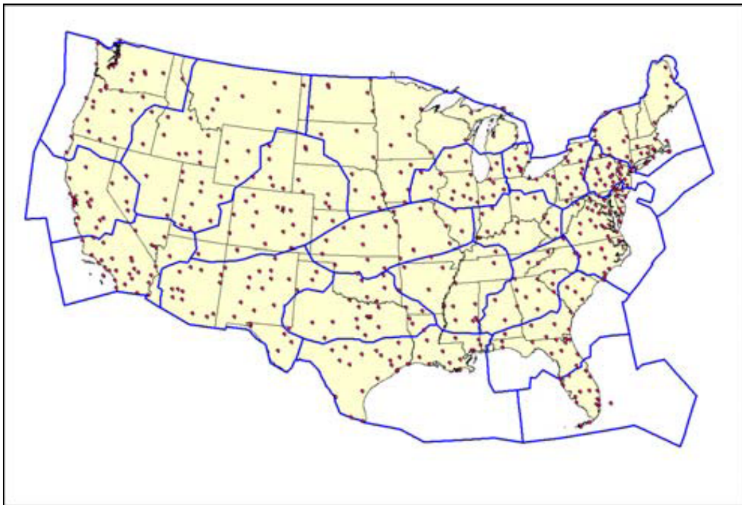
Figure 1. Current distribution of high altitude very high frequency omni-directional radio range (VORs) in the US by ARTCC Region (Laydon & Powell, 2003).
