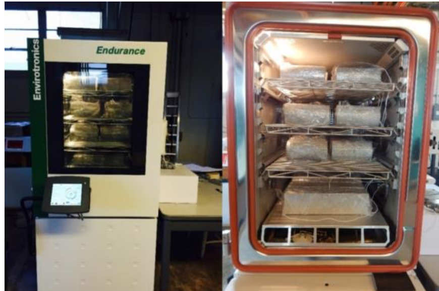
Figure 3-1: Environmental chamber and samples placed in environmental chamber for freeze-thaw exposure regimen
