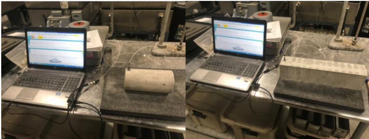
Figure 3-5: Experimental setup for resonant frequency test in transverse mode: cylindrical specimen and prism specimen
