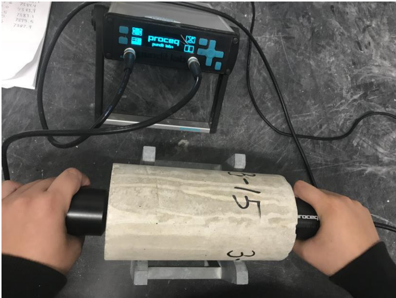
Figure 3-6: Experimental setup for ultrasonic pulse velocity test
