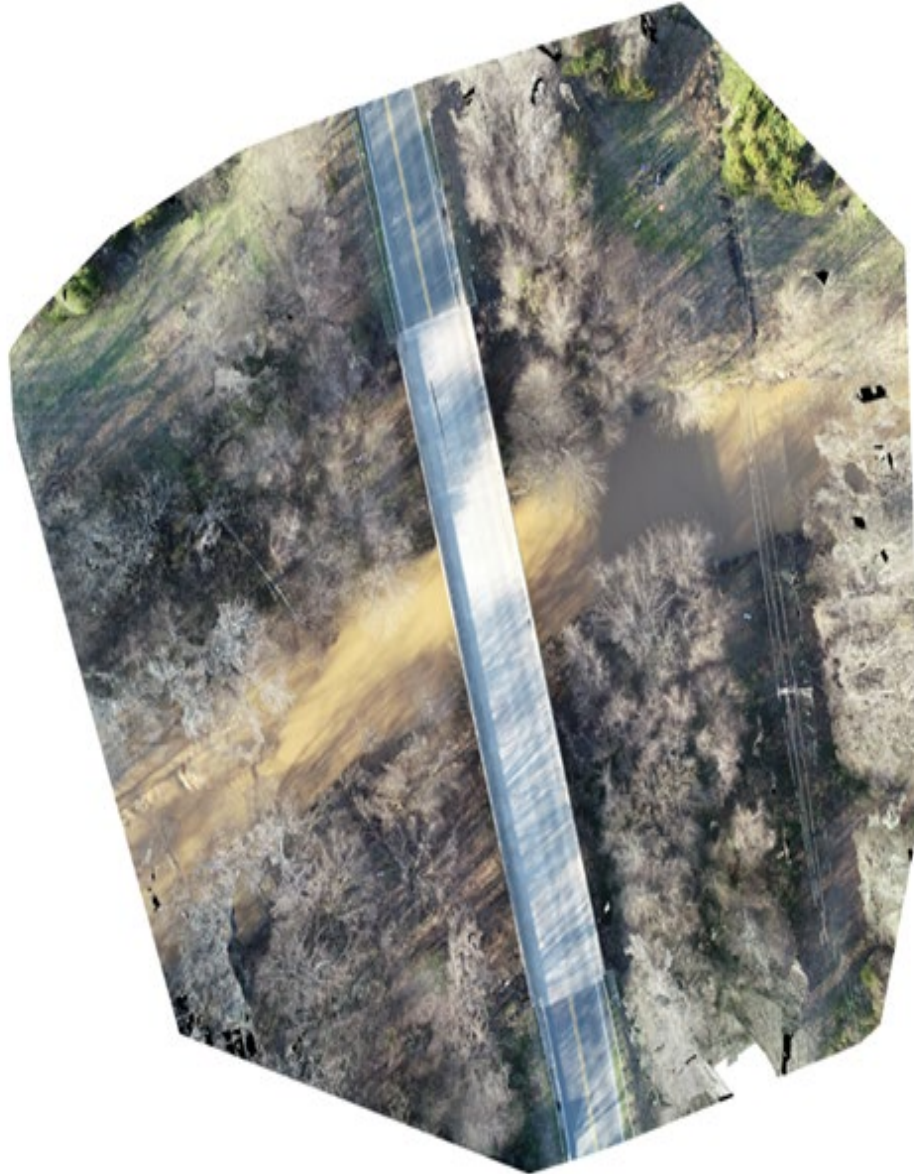
Figure 3.8. Orthomosaic (with 3D information) generated using SfM technique for Site #16 (see Table 3.1 for site information).
