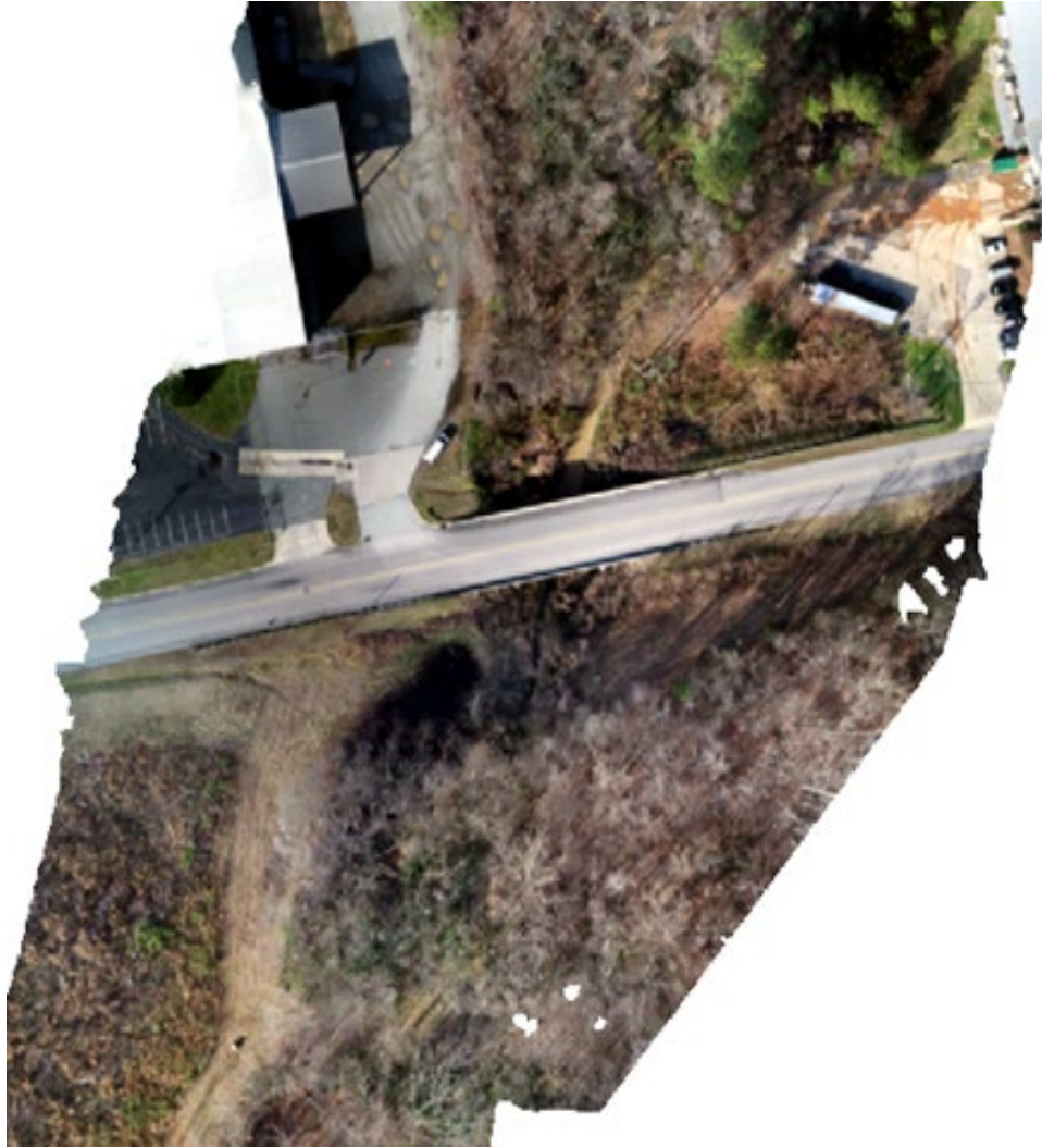
Figure 3.5. Orthomosaic (with 3D information) generated using Structure from Motion technique for Site #5 (see Table 3.1 for site information).
