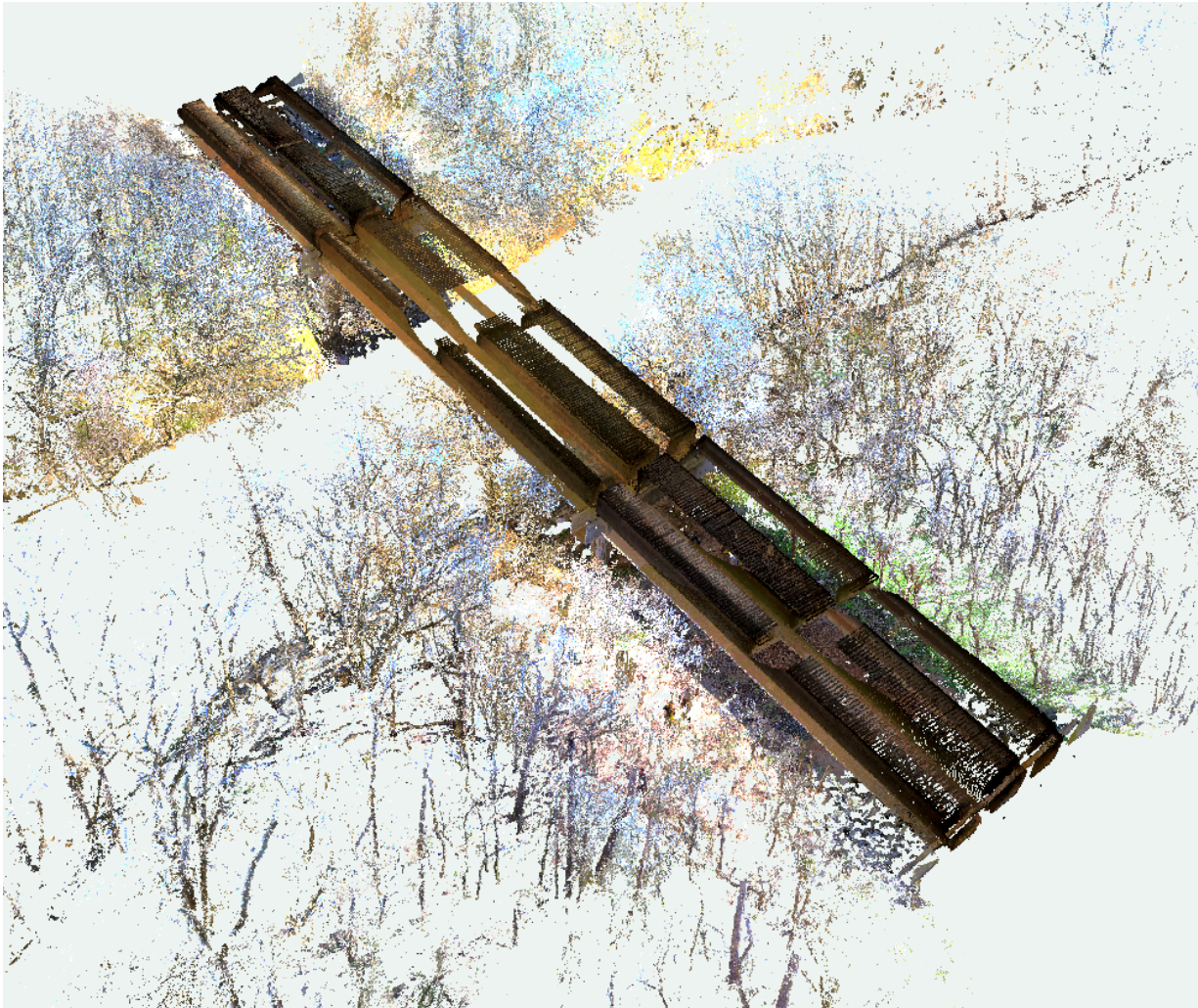
Figure 3.2. Illustration of collected LiDAR point cloud (Site# 16, stitched from two scans with a total of 147,166,173 points; see Table 3.1 for 2D image of the site).
