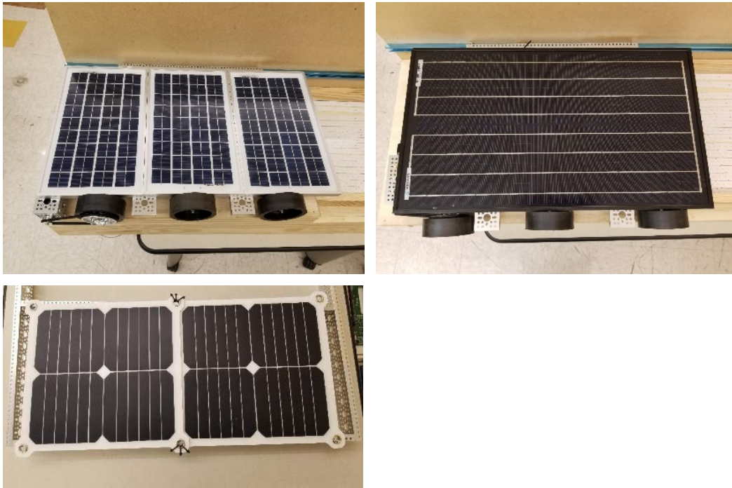
Figure 18. Three solar panels frames constructed for lab-scale prototype.
