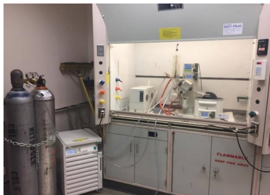
Figure 32: Recovery of asphalt binder (rotavapor)
