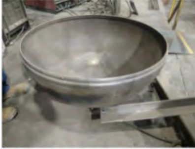
Figure 12. Photograph. View of a typical tank head.
