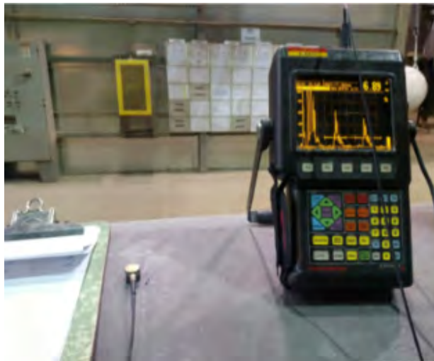
Figure 8. Photograph. Handheld Panametrics Epoch 4 unit used for the calibration tests - complete unit showing transducer.
