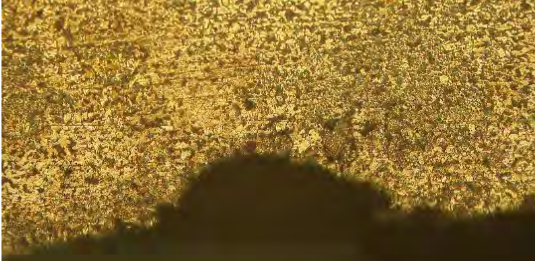
Figure 36. Image. Optical microscopy view of cross section across the region of the MP crack indication.
