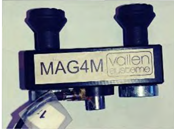
Figure 44. Photograph. Magnetic holder used in AE monitoring.
