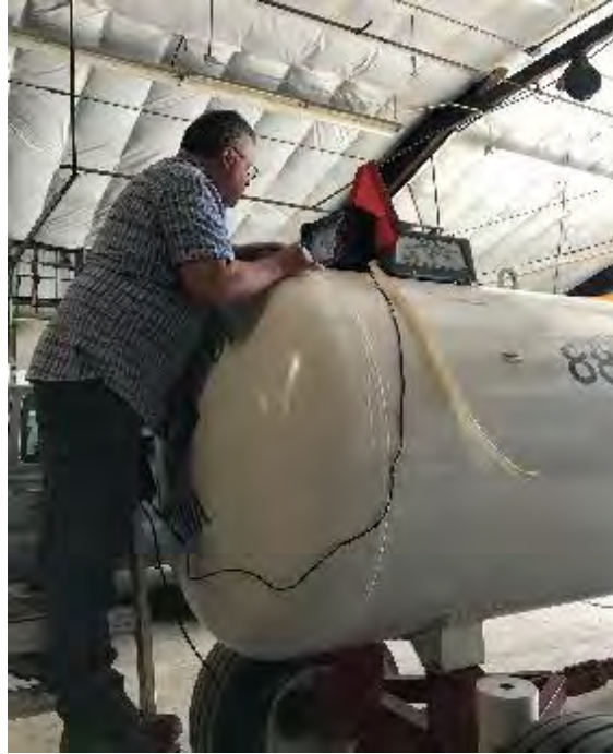
Figure 20. Photograph. Post-hydro ultrasonic examination of suspected crack growth/nucleation sites.
