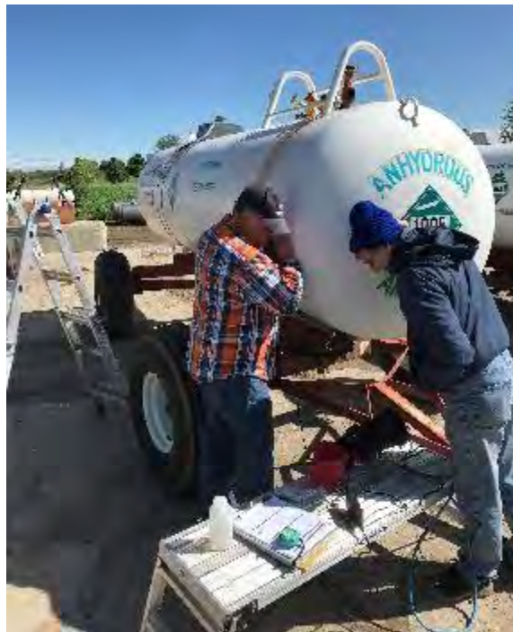
Figure 13. Photograph. Testing of the end cap weld.
