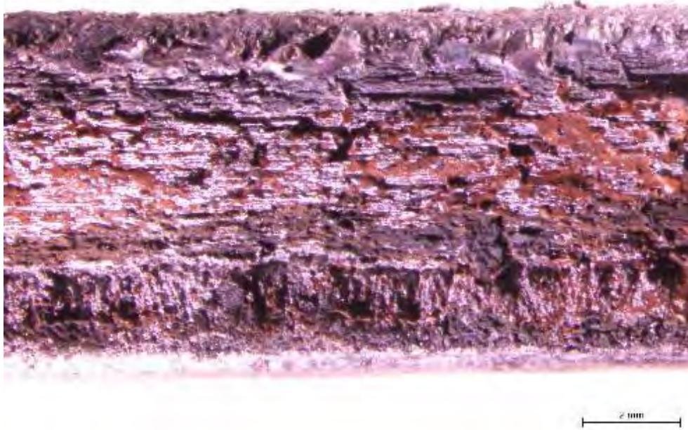
Figure 38. Image. Stereoscopic view of section 3 through-crack.
