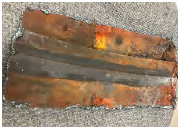
Figure 29. Photograph. Section 4 from tank #8161, before cleaning.
