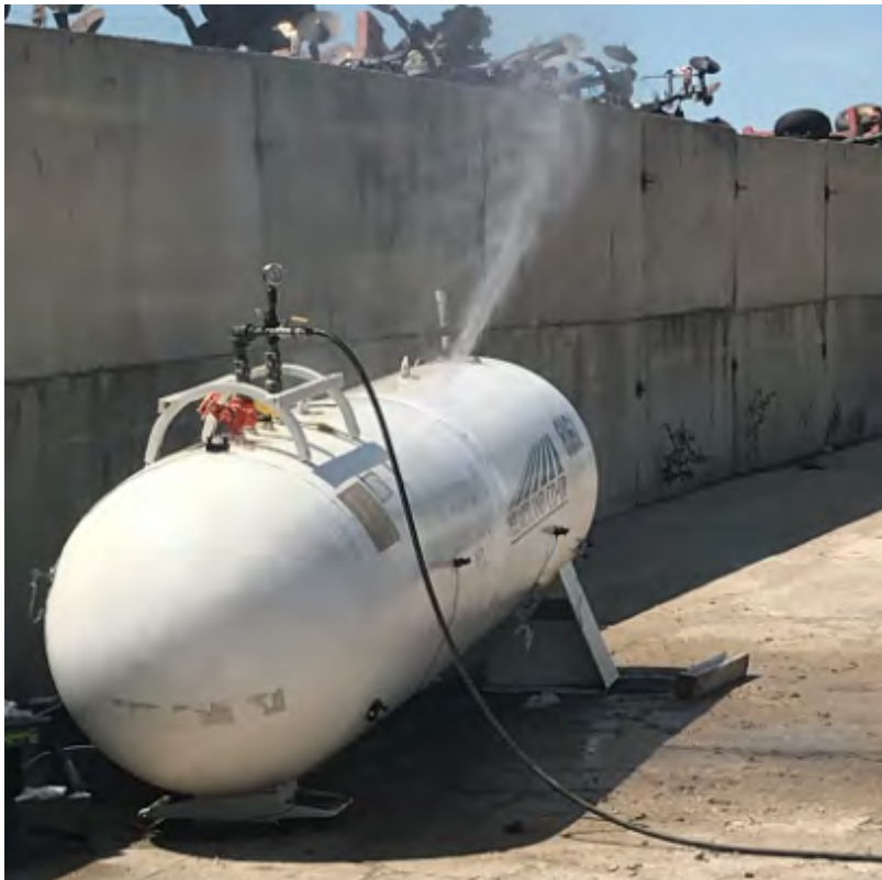
Figure 21. Photograph. Tank #8161 tested to failure.
