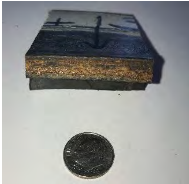
Figure 37. Photograph. Macroscopic view of section 3 through-crack.
