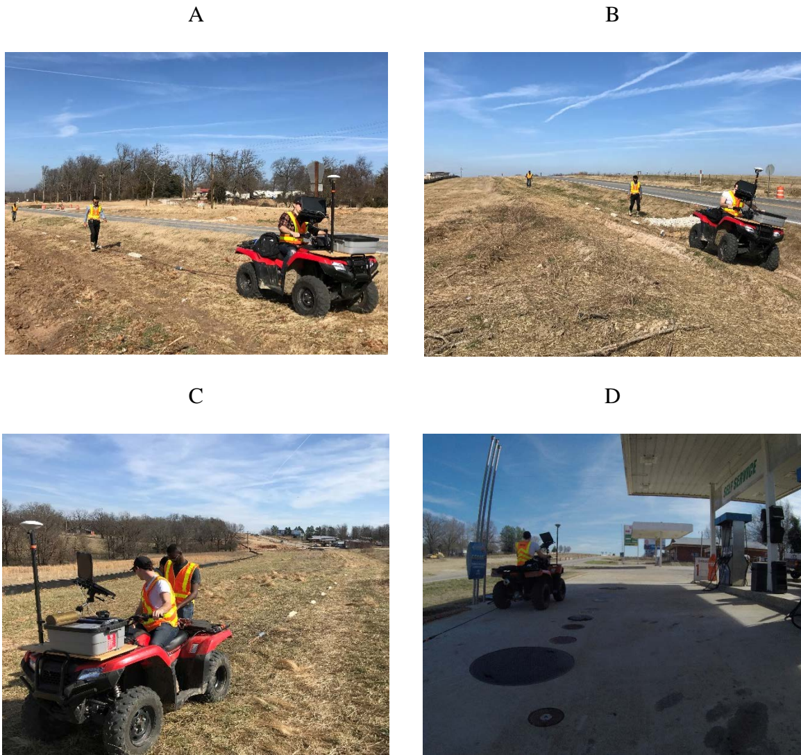
Figure 3-10. Along the Alpena Highway alignment OhmMapper towed at; A) STA 403+00 right side of highway, B) STA 451+00 passing over a buried utility crossing the highway on the right side, C) STA 484+00 left side of the highway, D) STA 491+00 passing through a gas station on the right side of the highway.
