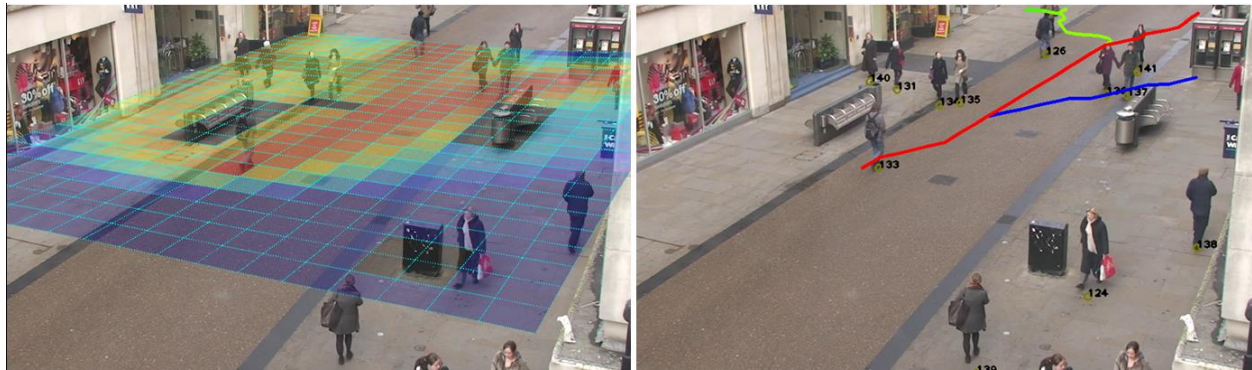
Fig. 4. Sample predictions. A map of expectation of future visitation (left) and specific paths ranked according to probability (right) are shown. The colors indicate probability, going from red (high) to blue (low).
