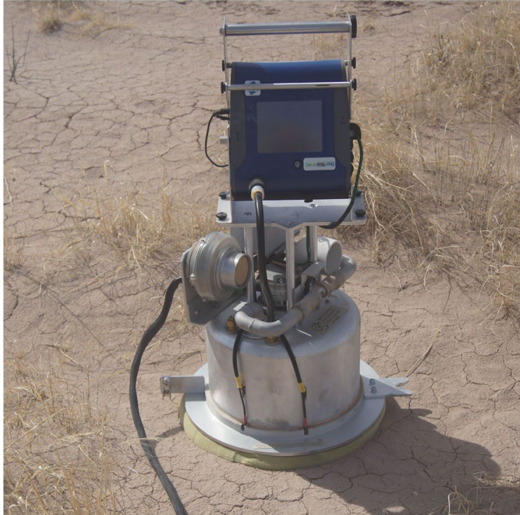
Figure 8. PI-SWERL in test configuration on Lordsburg Playa undisturbed surface with polygonal crusts.
