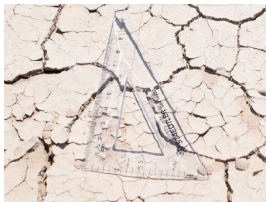
Figure 20. Polygonal surface crusts on playa showing highly erodible, wind-entrainable material exposure beneath the crusts where they are broken, removed, or disturbed.
