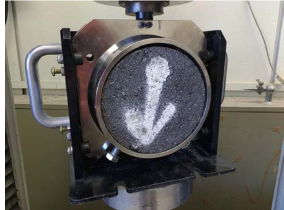
FIGURE 9 – Bond Shear Strength Tester.
