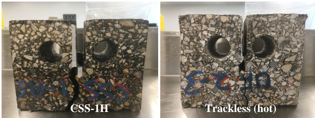
Figure 4-10. Reflection Cracking through Different Sample Types.
