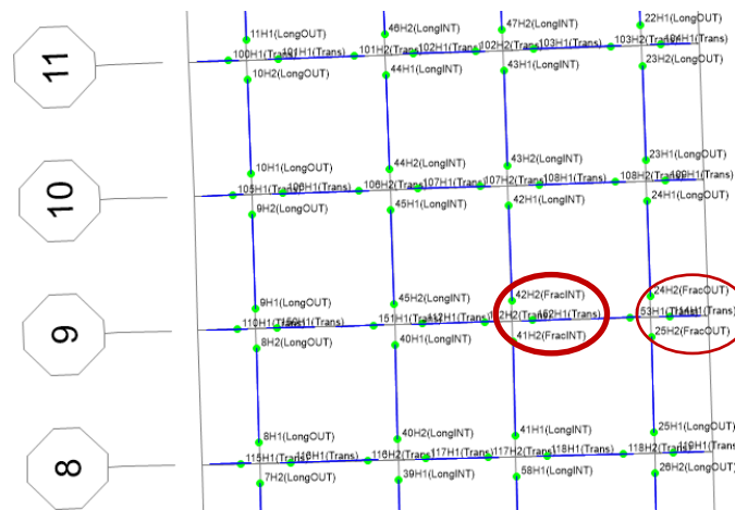
Figure 4.11. Fractured Hinge Pattern.
