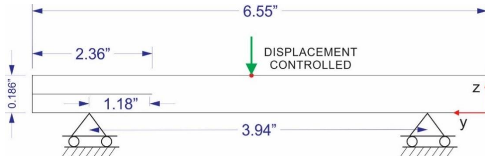
Figure 53. ENF experimental geometry and BCs
