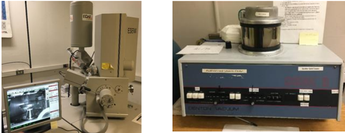
Figure 126. SEM imaging equipment (a) XL30 ESEM FEG (b) Sputter coater
