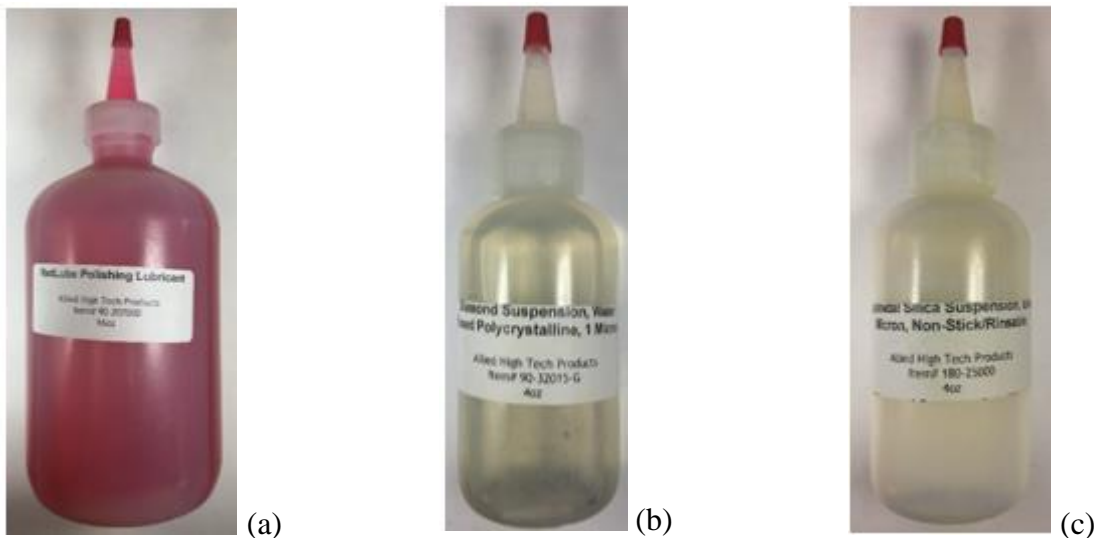
Figure 124. Polishing materials (a) RedLube (b) Diamond suspension (c) Colloidal silica suspension
