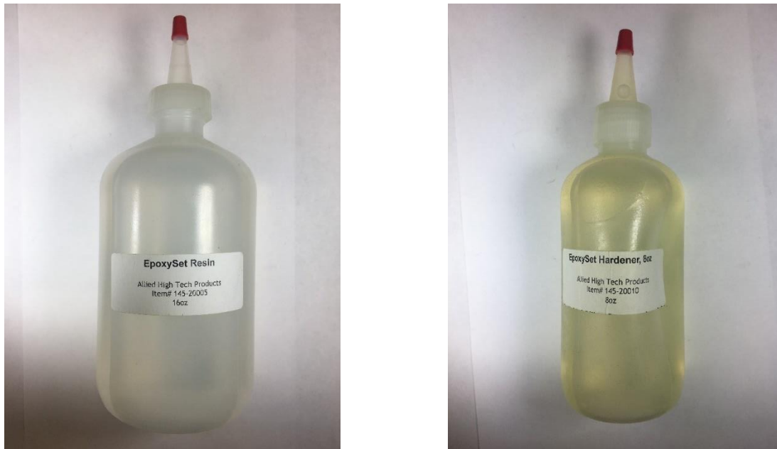
(a) (b) Figure 121. Epoxy set components (a) Resin (b) Hardener
