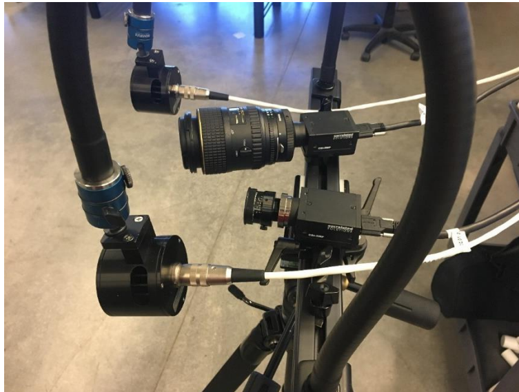
Figure 34. Typical camera setup for ENF and DCB tests, Tokina 100 mm lens (top) and Schneider 35 mm lens (bottom)
