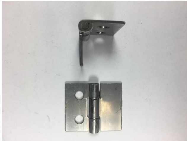
Figure 32. Piano hinges for DCB test
