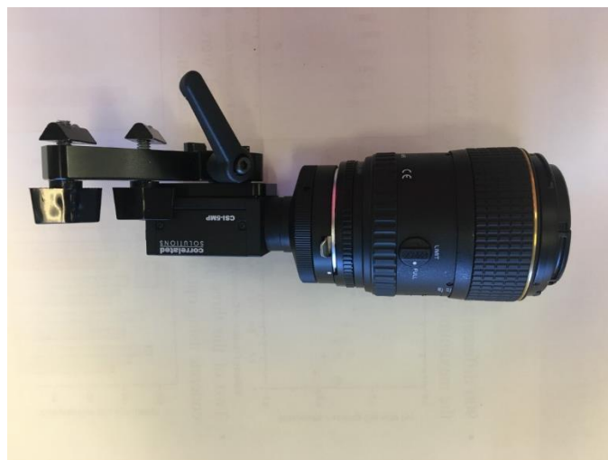
Figure 35. Tokina 100 mm lens on Point Grey Grasshopper 3 camera
