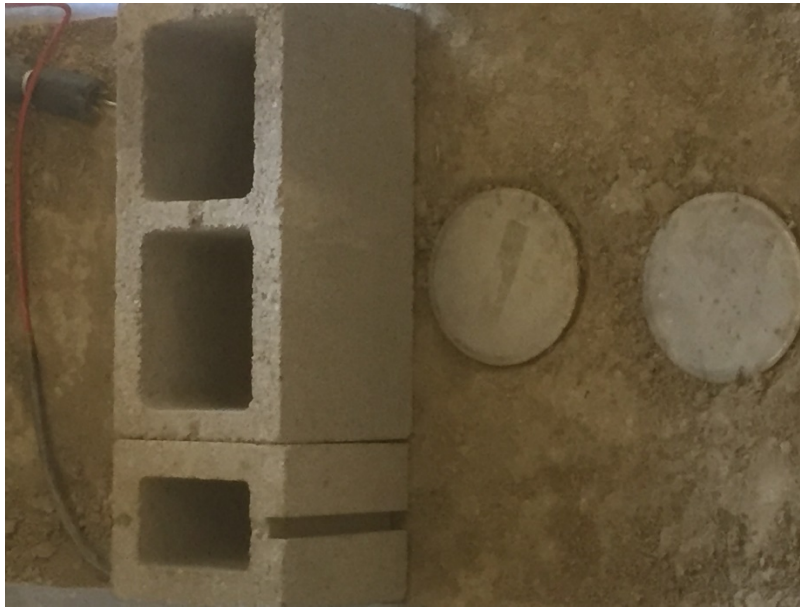
Figure 40. Install vertical pressure cells at the wall base
