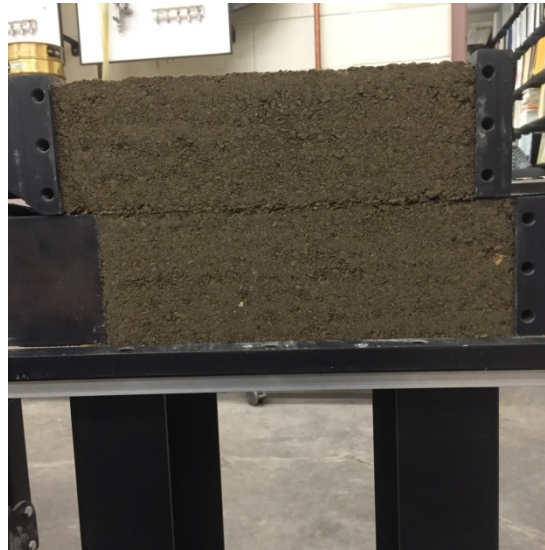
Figure 25. Backfill with geosynthetic inclusion after shearing
