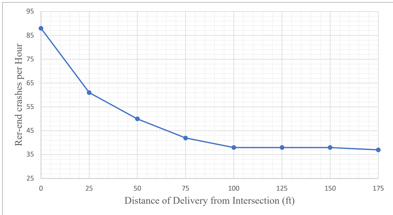
Figure 0.8. Effect of a bus curbside stop location on the number of rear-end conflicts
