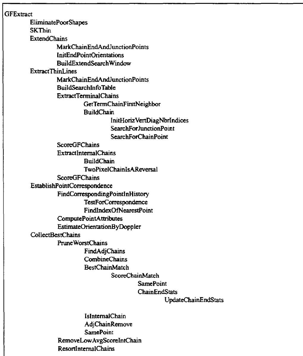
Figure 44. Function call tree for the gust front extraction phase of MIGFA (see text for description).
