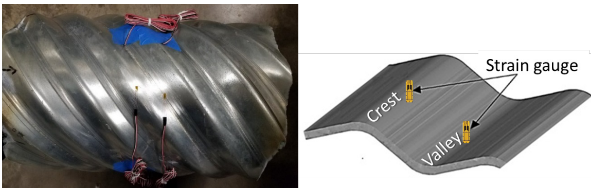
Figure 3.5: Strain gauges at both the crest and valley of a corrugation in the transversal direction of the pipe
