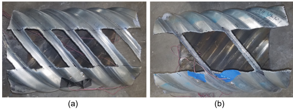
Figure 3.3: Corrugated Steel Pipes with Simulated Corrosion: (a) 50% Cutout and (b) 90% Cutout
