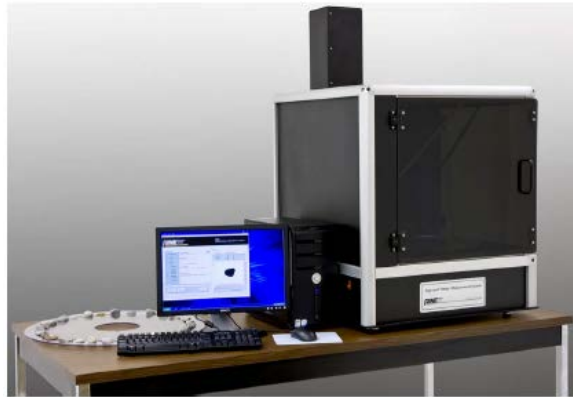
Figure 6 - AIMS2 equipment and set-up (Gates et al. 2011)
