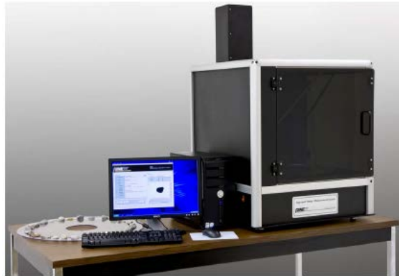
Figure A-31 - AIMS2 equipment and set-up (Gates et al. 2011)
