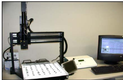
Figure A-30 - AIMS1 equipment and set-up (Gates et al. 2011).
