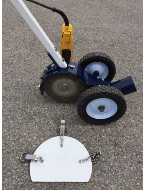
Figures 8. Second prototype device, side cover removed
