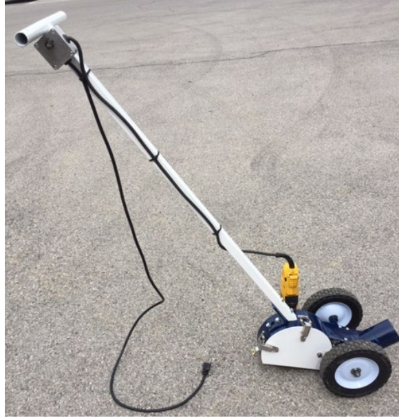
Figure 7. Second prototype bridge joint cleaning device
