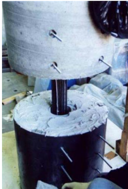
Figure 2-5: Application of epoxy at interface between column segments used by Hewes and Priestley (2002)
