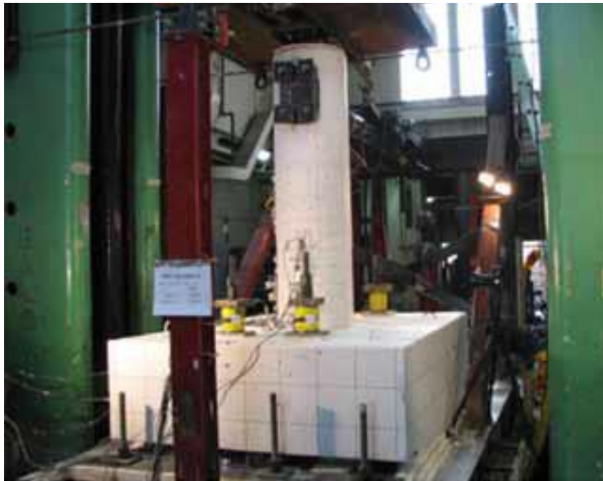
Figure 2-26: Testing of the column – bent cap connection by Pang et al. (2008)
