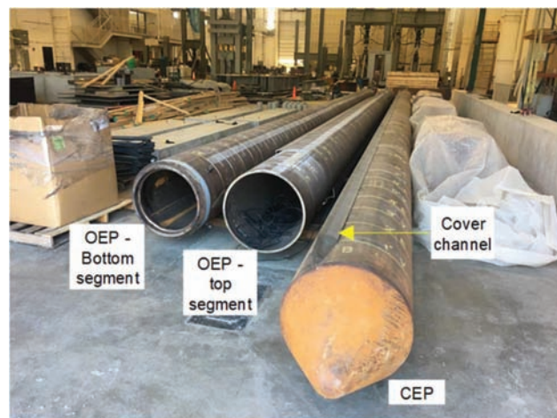
Figure 3.4 Closed-ended test pile and open-ended test pile (top and bottom segments) with instrumentation completed. (Modified after Han, Ganju, Salgado, & Prezzi, in press b.)
