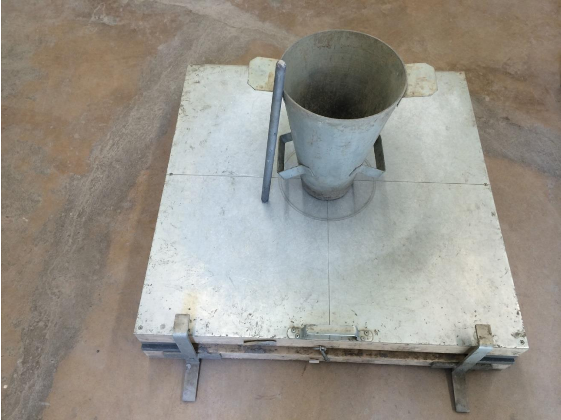
Photo B-2: ASTM C 1611 "Standard Test Method for Slump of Self-Consolidating Concrete" "Spread-Test"
