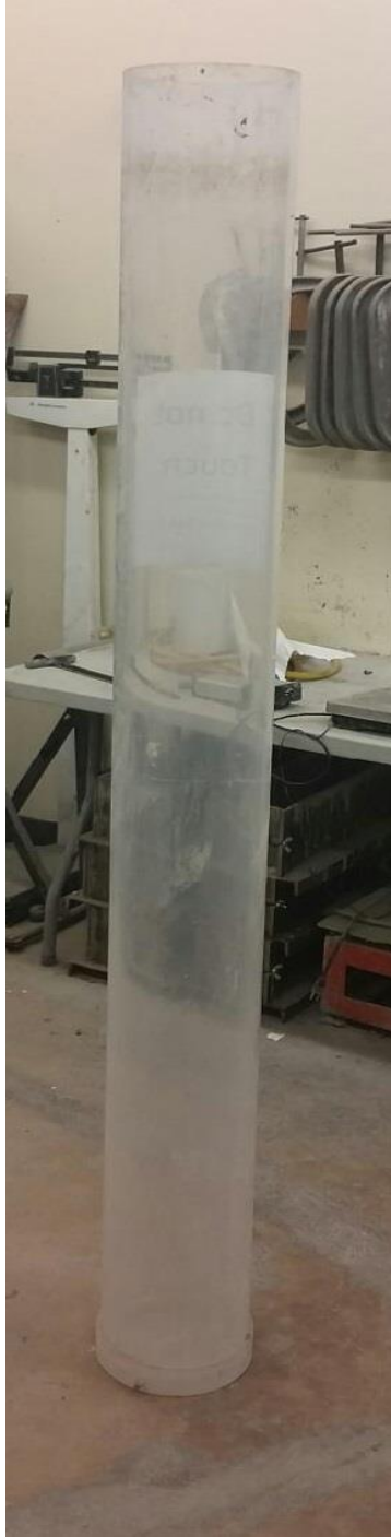
Photo B-3: US Army of Engineers Standards CRD-C 61 – 89A “Test Method for Determining the Resistance of Freshly Mixed Concrete to Washing Out in Water”
