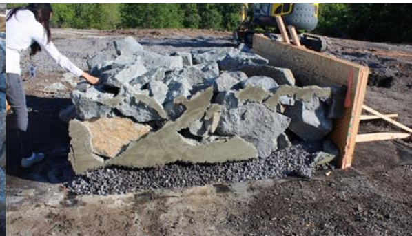
Photo 14 Grout Settlement at the Bottom
