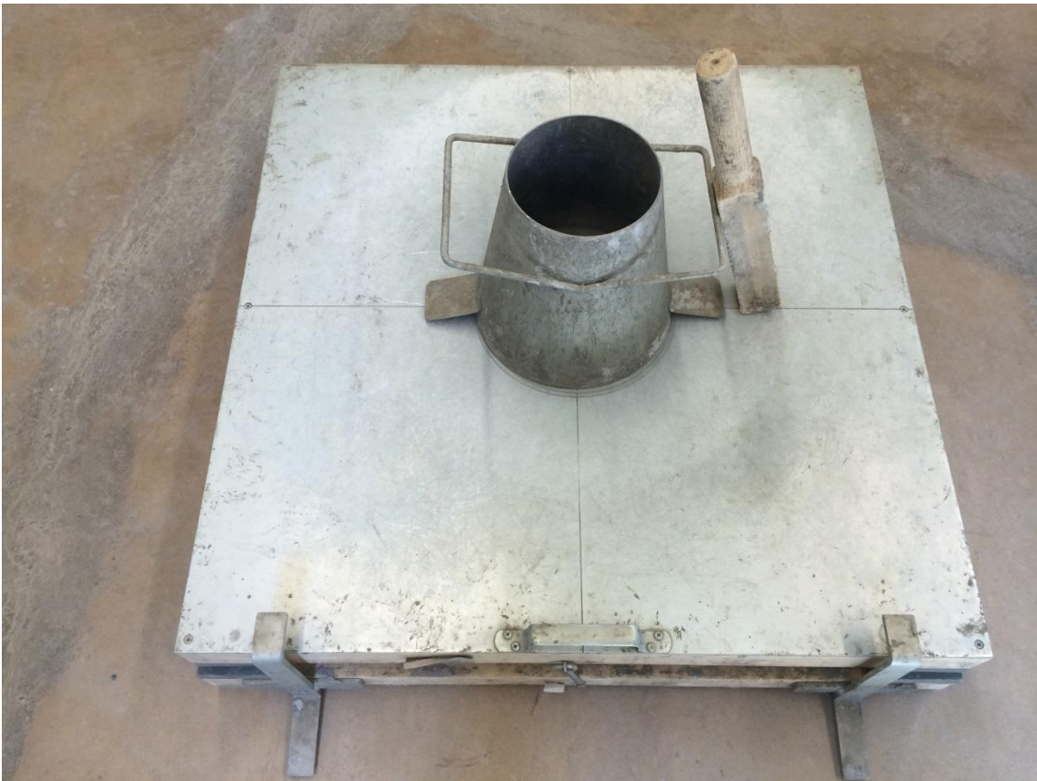
Photo B-1: European Flow Table Test “Tap-Test”
