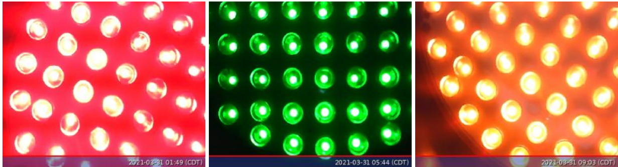
Figure 24: Lawrence field test data collected in March 2021 after the field visit on Feb 25 th to fix those two problems of the remote data monitoring system, showing the normal performance of the red, yellow, and green signal lights under spring weather conditions, especially for the green signal light which had the longest power-on time. The ambient temperature was slightly lower than that on the yellow and red signal lens with short power-on time.
