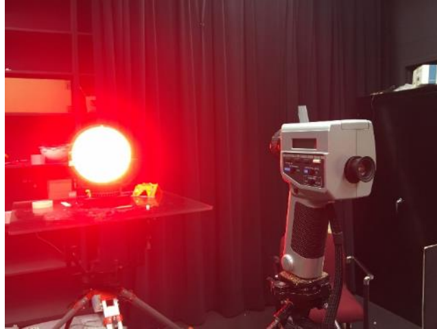
Figure 10: Lab measurement of the signal lens surface luminance using the code recommended measurement method with a luminance meter.
