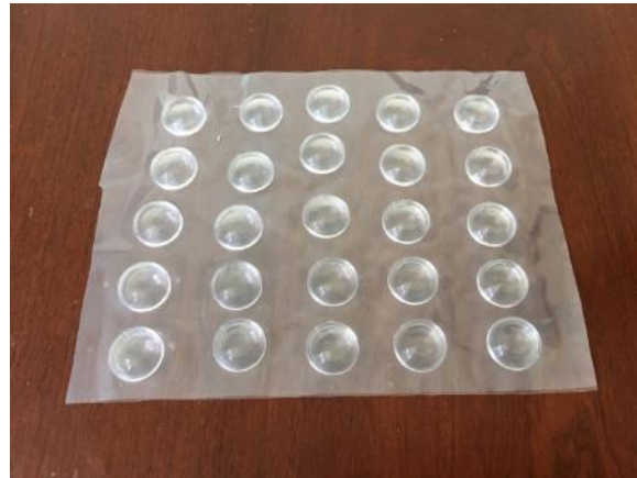
(d) Fresnel lenses (diameter: 15 mm, focal length: 11.5 mm, thickness: 1.5–2.0 mm)
