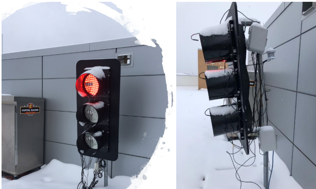
Figure 13: Prototypes of the new type of self-de-icing LED signals (Red, Yellow, Green) for highway signalized intersections, and their performance and reliability tests on the roof of the University of Kansas engineering complex, powered by a real traffic control cabinet.
