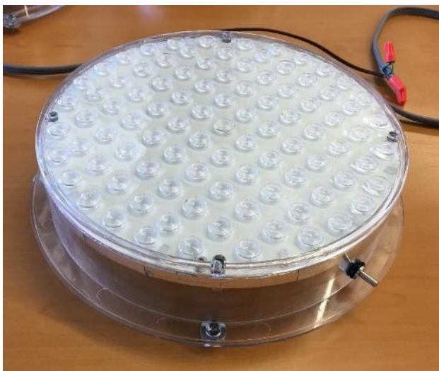
Figure 1: Prototypes of the new type of self-de-icing LED signals (Red, Yellow, Green) for highway signalized intersections
