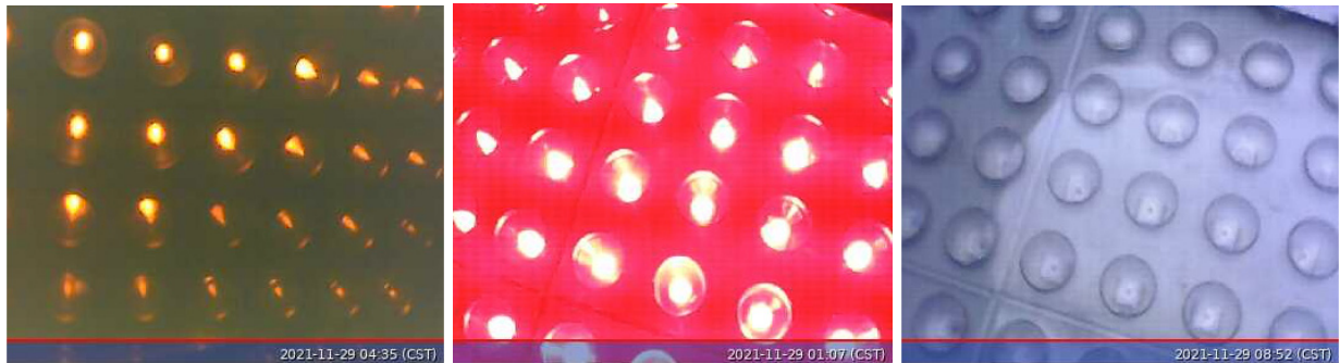
Figure 30: Michigan field test data collected in November 2021 after the field installation on November 4 th , showing the normal performance of the red, yellow, and green signal lights under mild and cold weather conditions. Note that before Nov 17, 2021, the green signal light had a higher lens surface temperature due to its longer power-on timing than the red signal light. This timing sequence was changed after Nov 17 per our request to keep the green and red signal with well-balanced power-on timing, resulting in close temperature measured on the lens surface for both green and red light.
