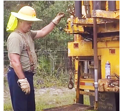
A technician has attached the VIP to a drill rod and prepares to lower it to the ground.
