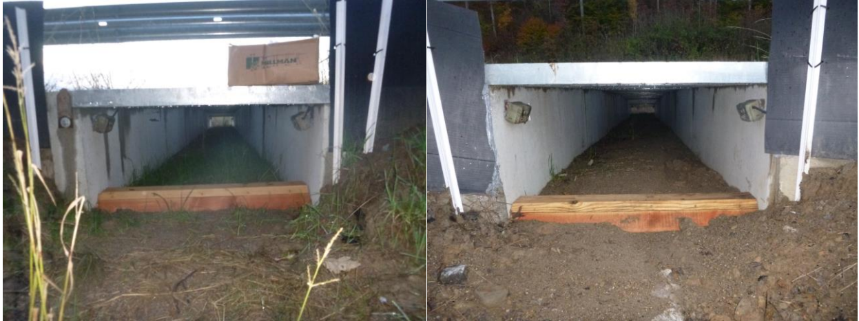
Figure A10-3. Spypoint Tiny-W3 cameras and viewing ramps set up to take photographs of the ecopassage entrances. Right photo shows some erosion from under the ramp after a rain, which was repaired later that day.
