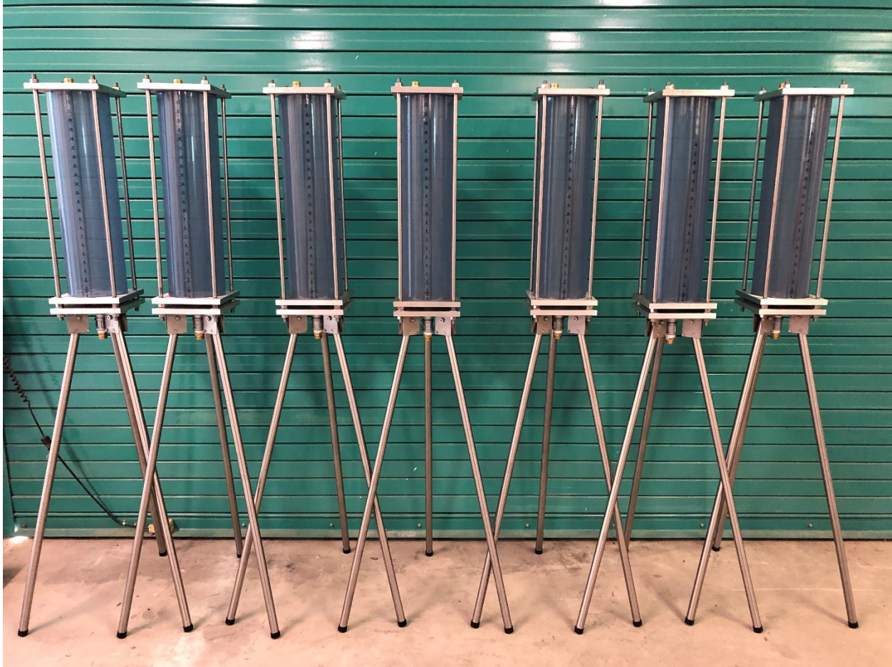
Figure 2-13. Seven new falling head vessels (prototype not depicted).
