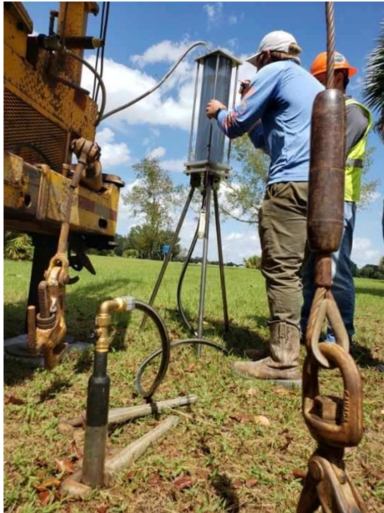
Figure 5-29. VIP being used for an infiltrometer tests.
