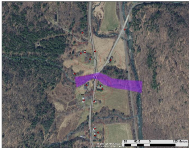
Figure 8. Illustration of 50m buffers around all residences within 300m of a transportation structure (Site 12a-10, Braintree).
