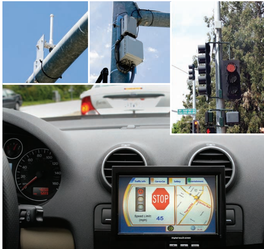
In California, this Test Bed demonstrates In-Vehicle Signal Information. Source: CalTrans and the PATH Program at the University of California at Berkeley.
