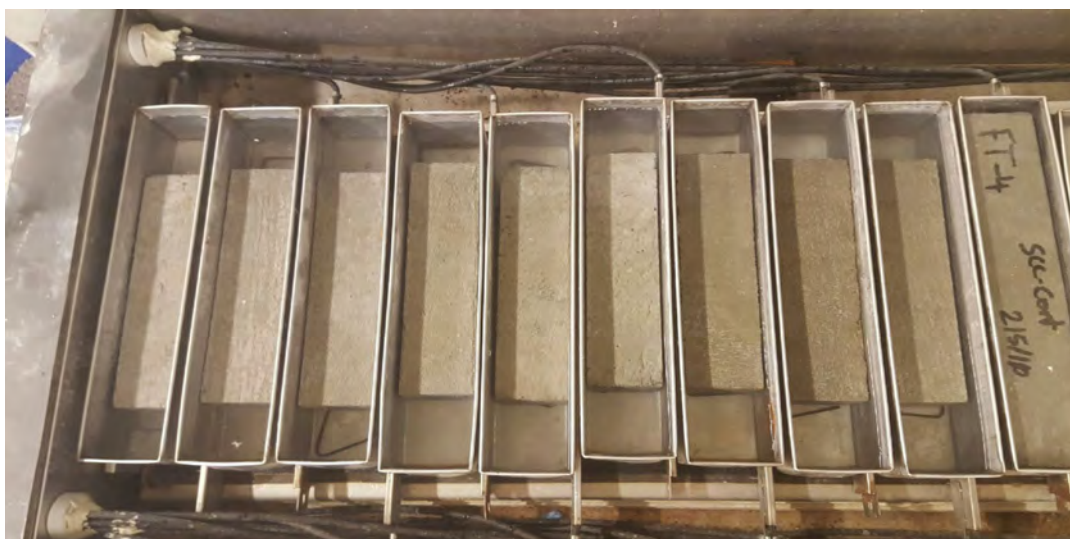
Figure 3.14. RCC specimens before the freeze-thaw test
