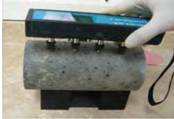
Figure 3.9. Testing apparatus for surface electrical resistivity of RCC
