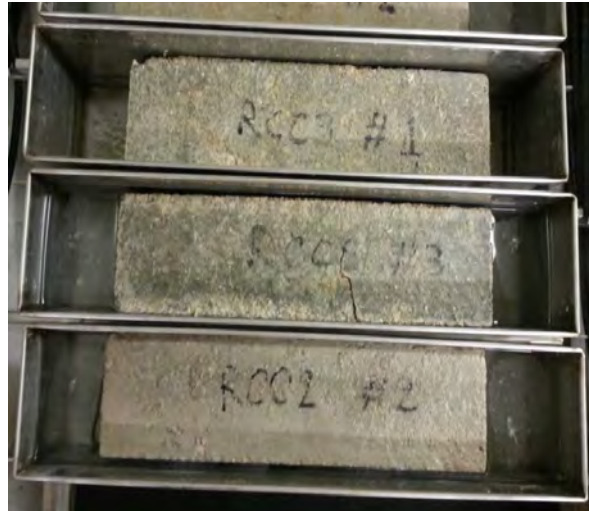
Figure 4.6. RCC specimens (RF mixture) cast in field after 30 freeze-thaw cycles (Khayat and Libre, 2014)
