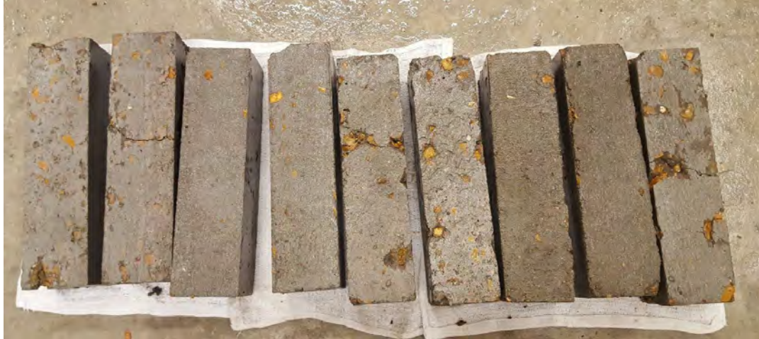
Figure 4.5. RCC specimens after 123 freeze-thaw cycles
