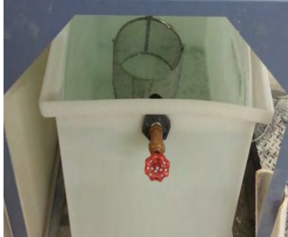
Figure 3.16. Apparatus used for measuring permeable voids in concrete
