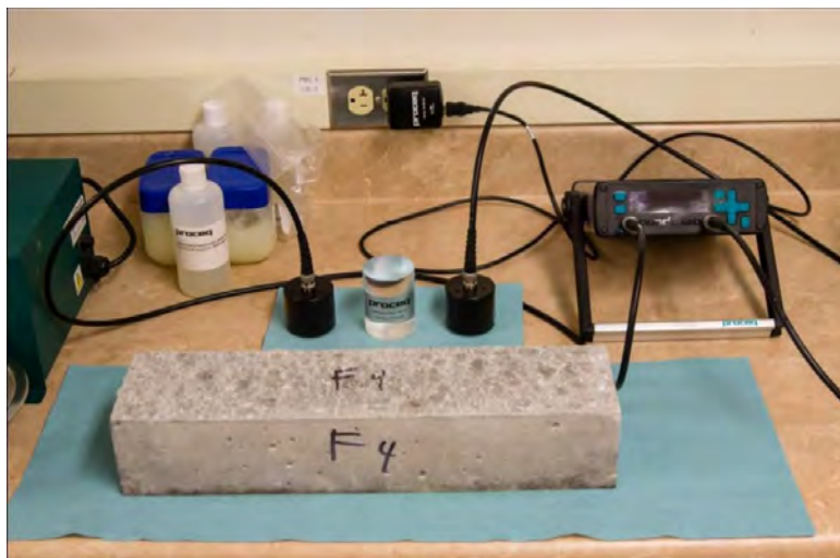
Figure 3.13. Testing apparatus for dynamic modulus of elasticity
