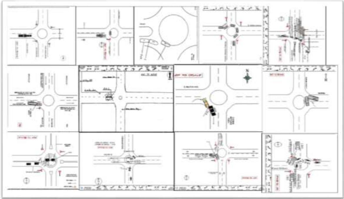
Figure E12.3 East/west bound road user at fault crashes at E Milton Ave./LA 92 at Chemin Metairie Rd. roundabout
