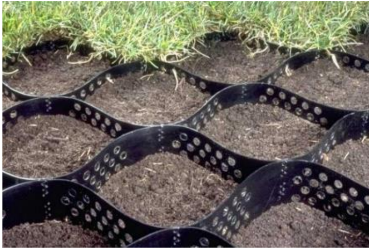
Figure 1.1 Geocell-confined soil (picture from prestogeo.com)
