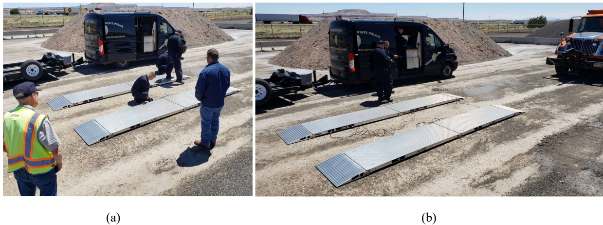
FIGURE 14 Weighing scale used to weight the test truck before and after filling it with sand. (a) scale installation. (b) scale after being wired.
