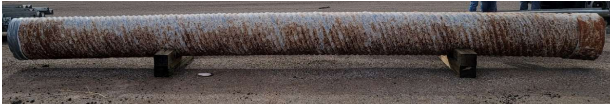
FIGURE 5 Corroded metal steel pipe
