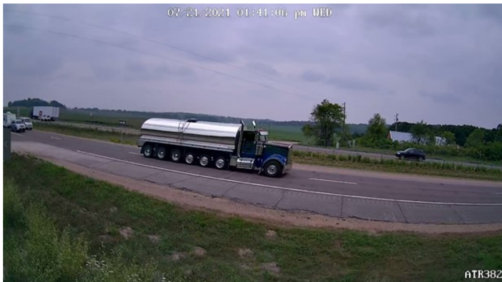
Figure 6.3 A tanker truck with lift axles on the road.
