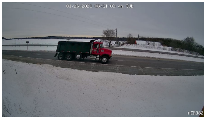
Figure 4.7 Vehicle #402283 – Class 6 (1/26/2021) Misclassified as Class 5.
