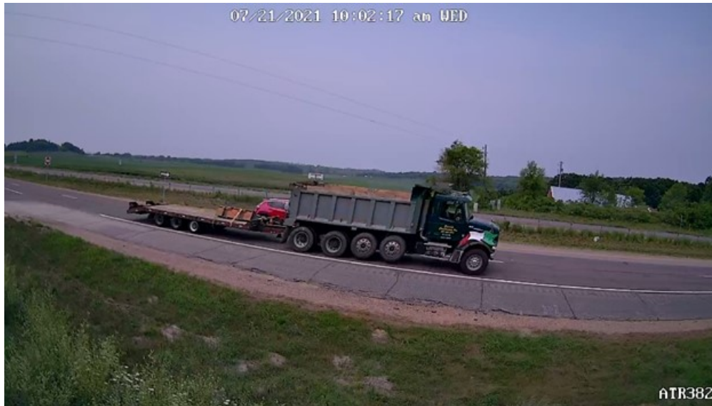
Figure 6.2 A dump truck with 2 raised lift axles pulling a trailer.
