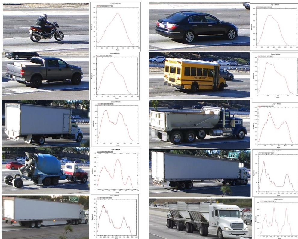
Figure 3.1 Loop Signatures for Different Type of Vehicles (Image from CLR Analytics Inc.).
