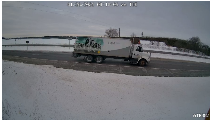
Figure 4.5 Vehicle #402197 – Class 6 (1/26/2021) Misclassified as Class 5.
