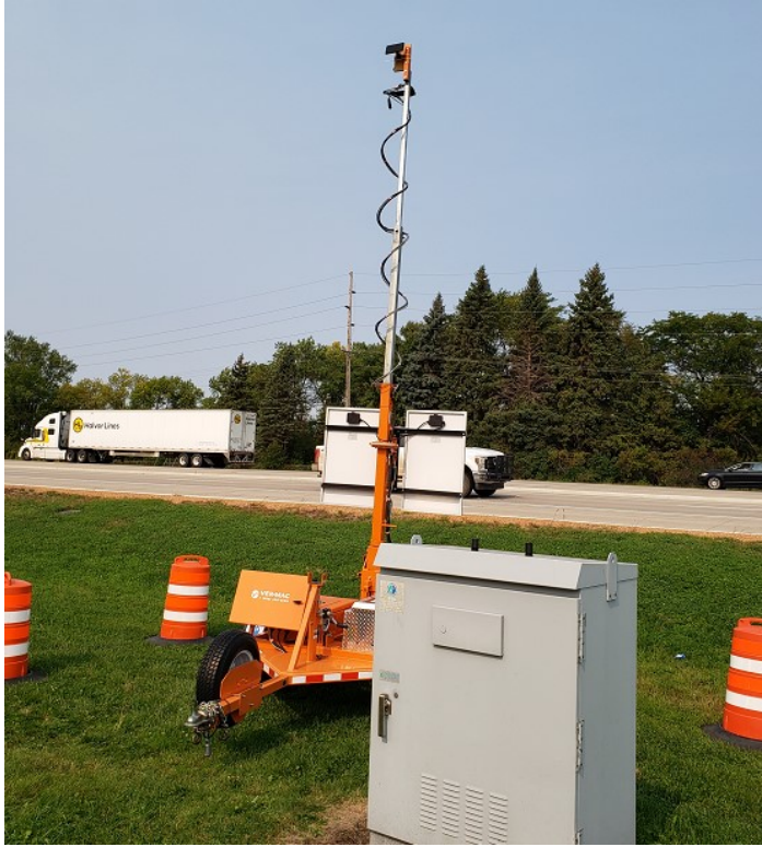
Figure 2.6 Image of a video data collection system mounted on a trailer next to ATR353 cabinet.
