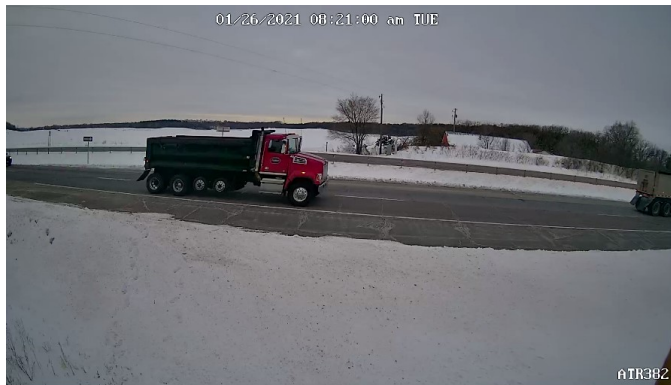
Figure 4.6 Vehicle #402282 – Class 6 (1/26/2021) Misclassified as Class 5.
