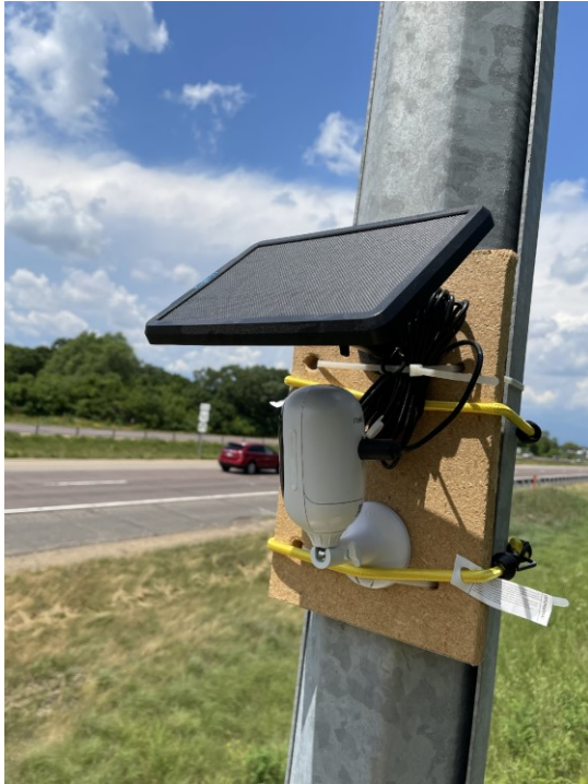
Figure 2.11 Image of a video data collection system mounted on a RTMC pole near ATR382.
