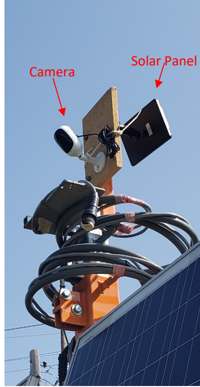
Figure 2.6 Image of a video data collection system mounted on a trailer next to ATR353 cabinet.
