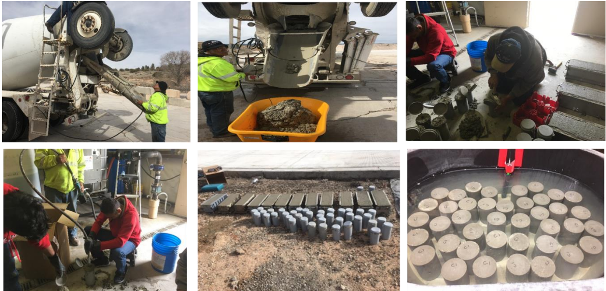
Figure 3.1. Cylindrical Specimens Preparation and Curing
