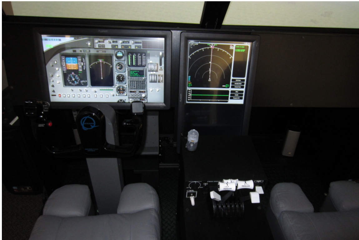
Figure 2. Two LCD Touch Screen Displays Inside the Cockpit. Yoke, Throttles and Flaps are also visible.
