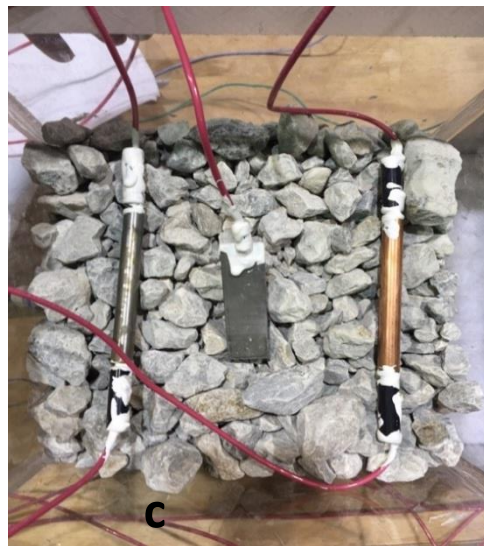
(a) Titanium plate electrical connection using bolt-screw mechanism and O-shaped terminal connector, (b) Final Electrodes setup in AASHTO Standard Material, (c) Final Electrodes setup in AASHTO No.57 Material
