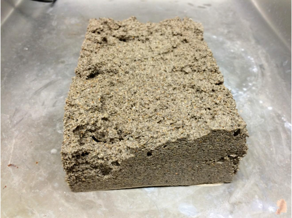
Figure 16: AASHTO Standard Gradation for RE Janes Material after 15 Hour Test is completed.
