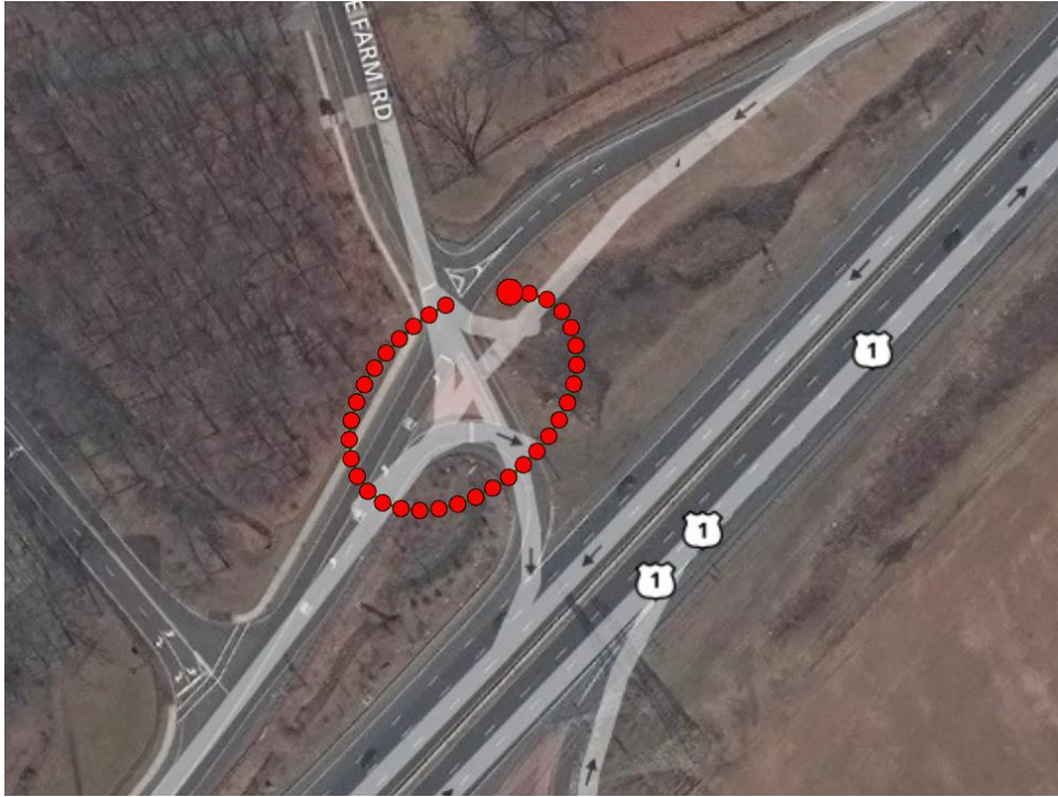
Figure 12: Circular Flight Pattern for 3-Dimensional Model Data
