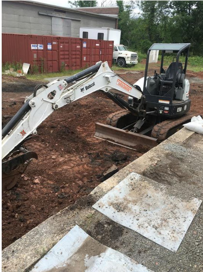
Figure 151: Bobcat E50 with 1ft (0.30m) bucket attachment
