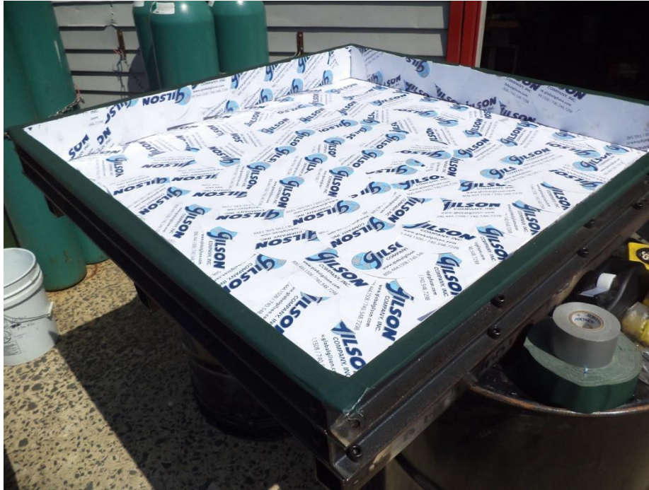
Figure 14: New 1 sq. m. asphalt compaction mold created in-house
