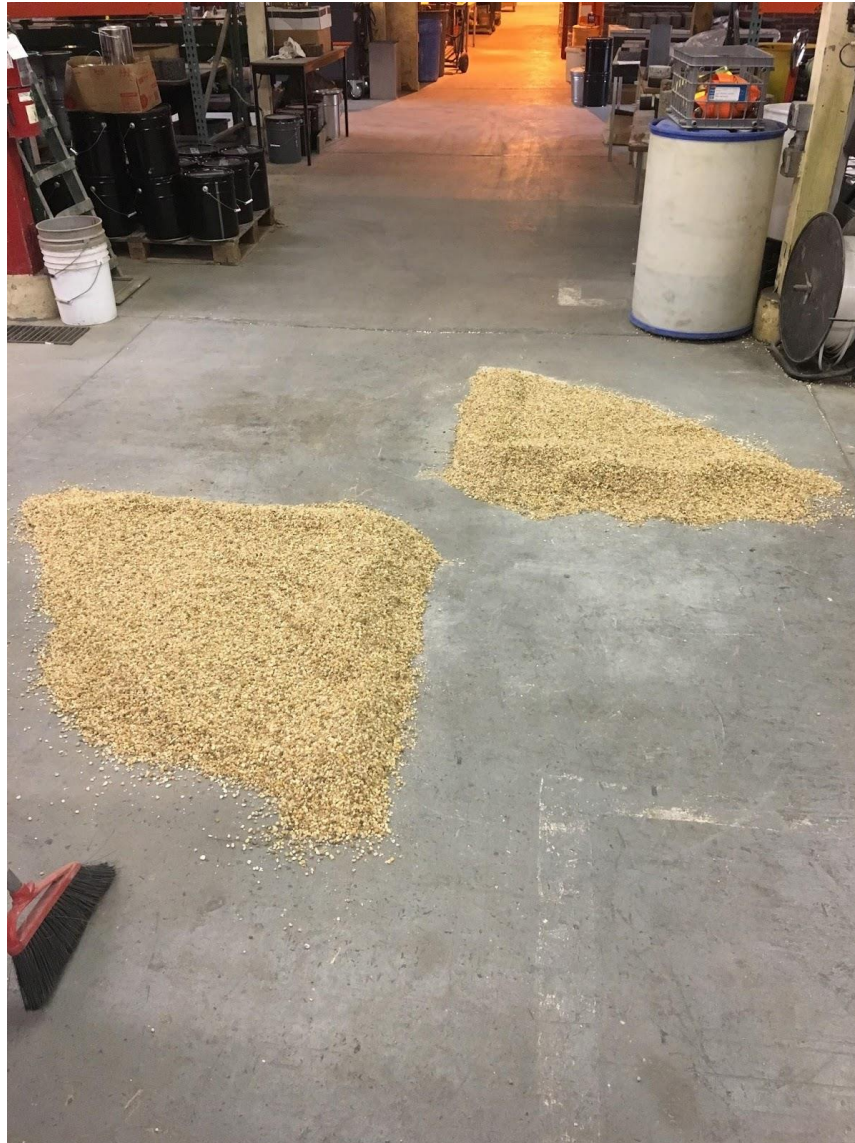
Figure 174: Quartering aggregate for sampling
