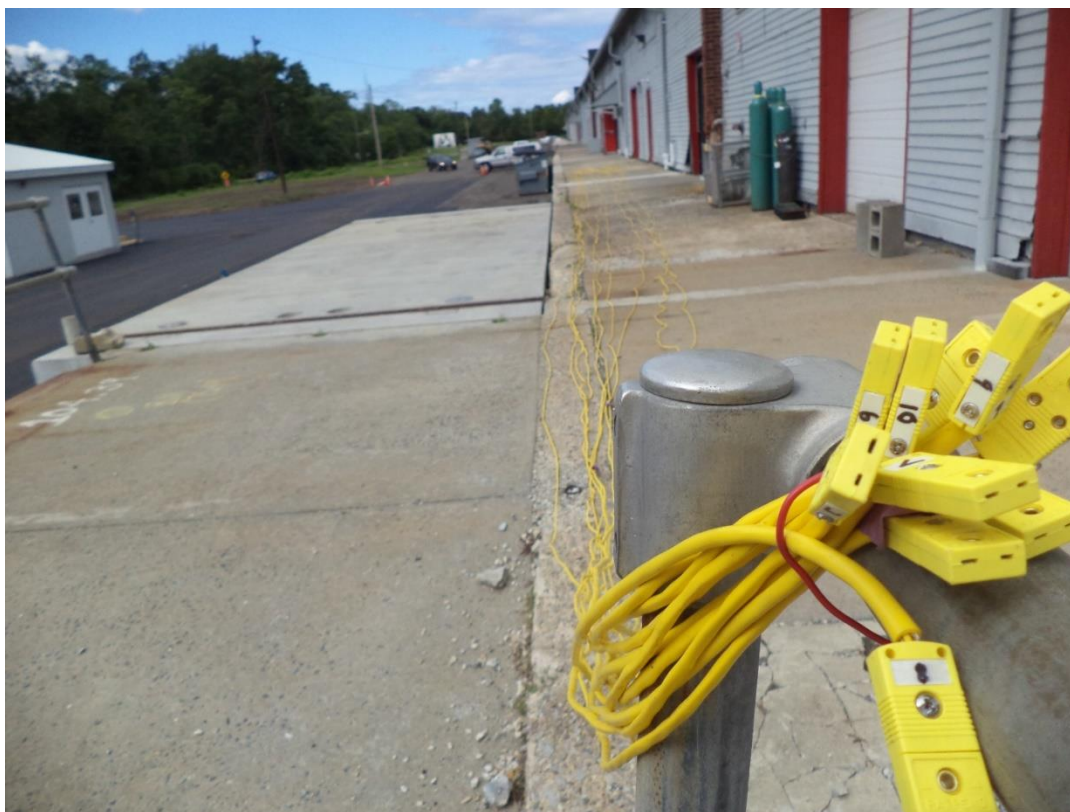
Figure 9: Preparing the thermocouple extension wire to be conjoined into a single probe
