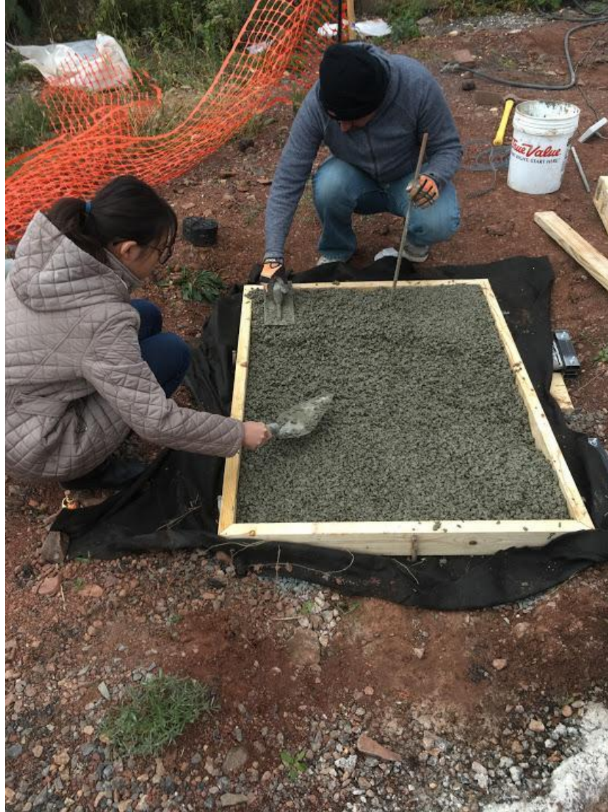
Figure 167: Hand work and rodding to create concrete field samples
