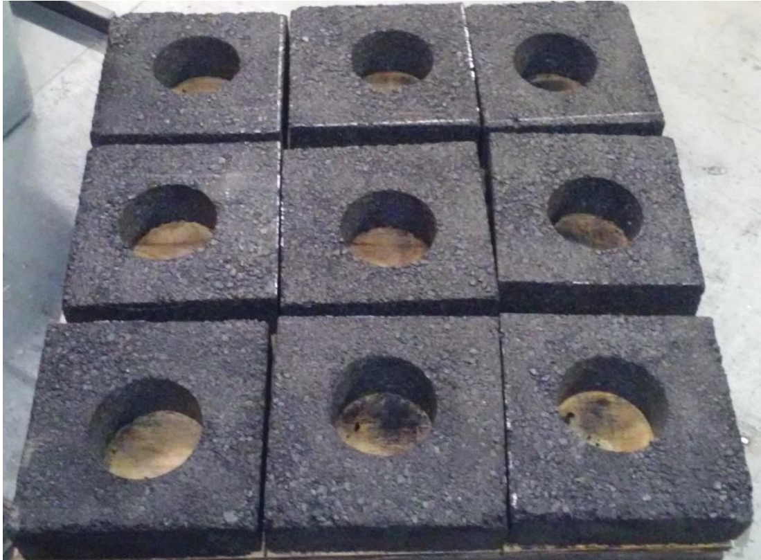
Figure 17: Asphalt verification slab utilized to practice compaction and verify the offset for the PQI380
