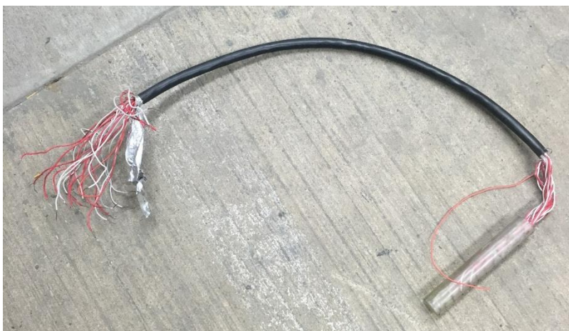
Figure 10: Initial J-Type thermocouple probe assembly
