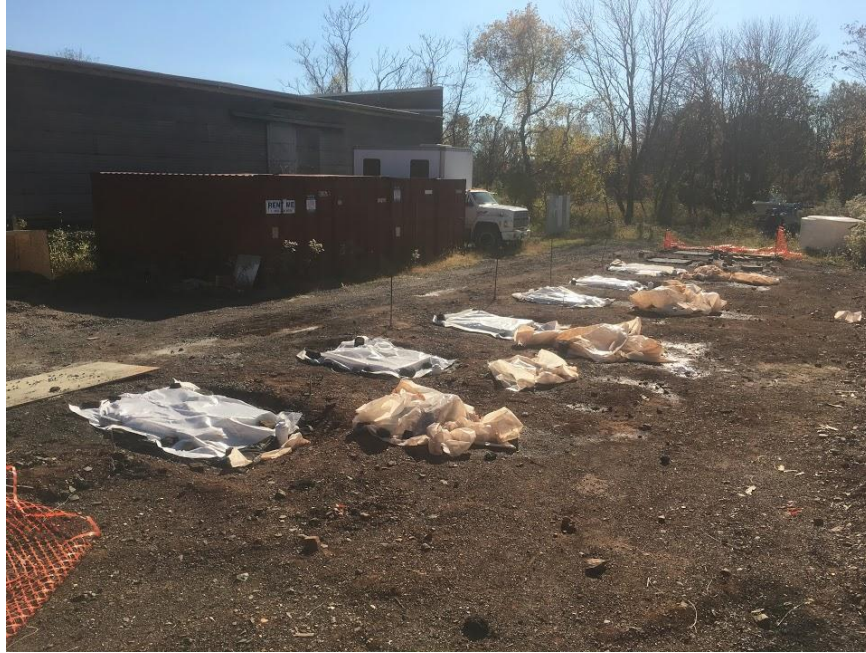
Figure 171: Prepared samples curing under plastic sheeting
