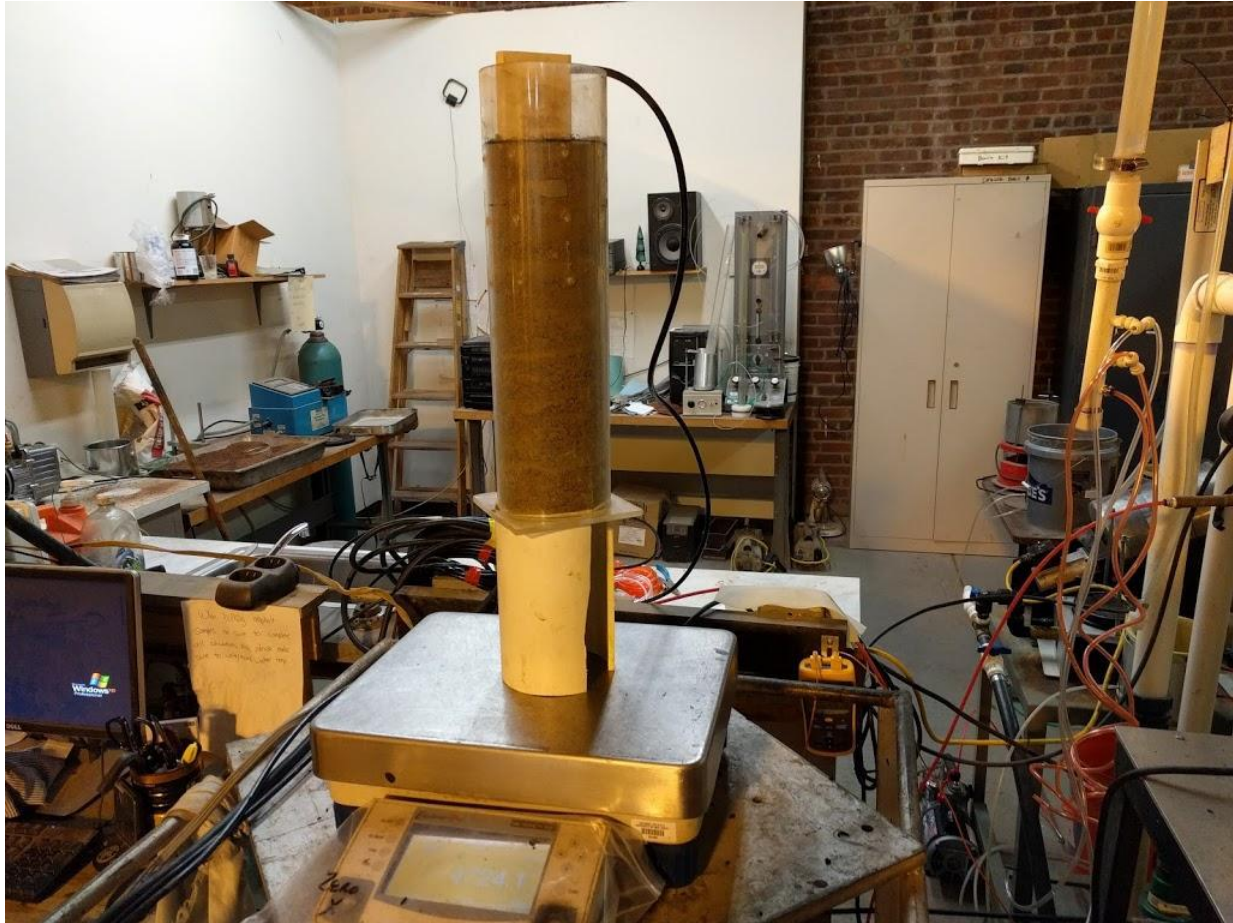
Figure 184: Dry TDR calibration sample, manifold is hanging on right after stemming from gravity fed bucket
