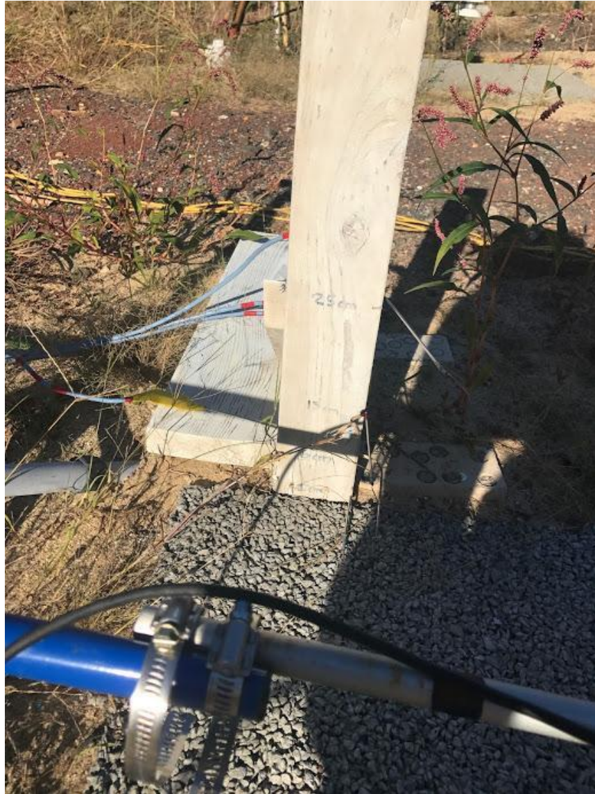
Figure 192: Type-E close proximity air column thermocouples
