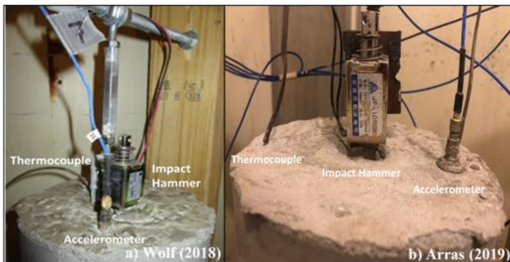
Figure 3.3 Seismic Modulus and Internal Temperature Monitoring
