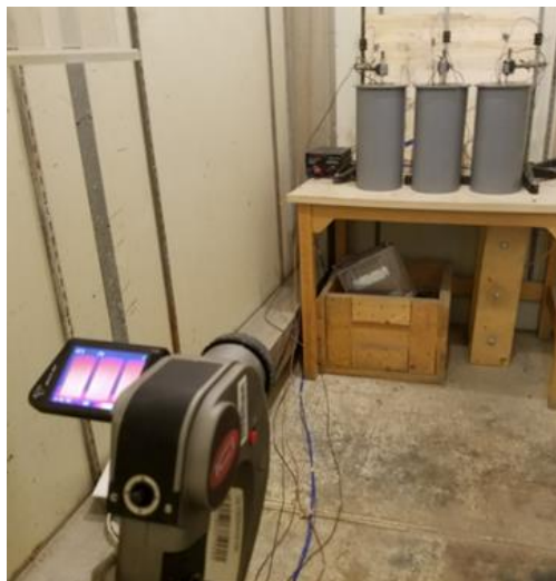
Figure 3.9 Set-up for Thermal Imaging of Cylinders
