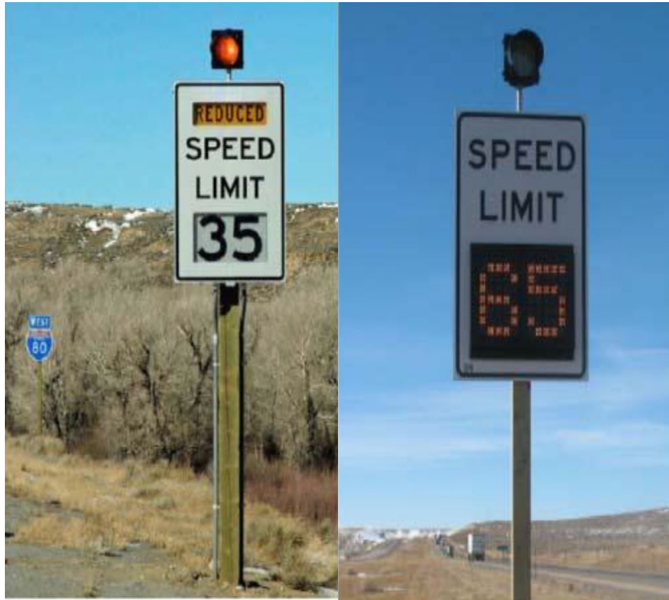
Figure 3.7 VSL Signs, Scrolling Film Technology (left) and LED Technology (right)
